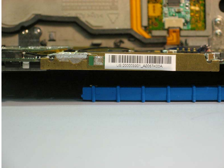
WiFi diversity antenna in front of unit
