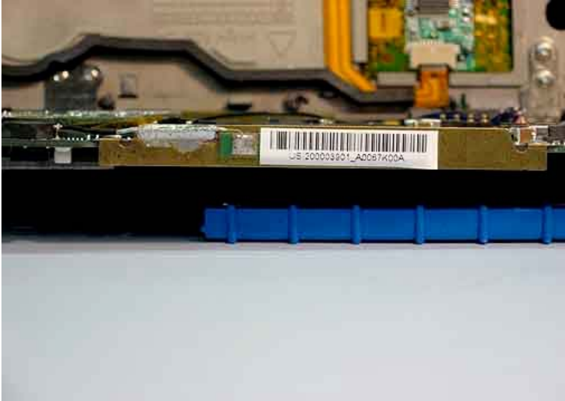
WiFi diversity antenna in front of unit
