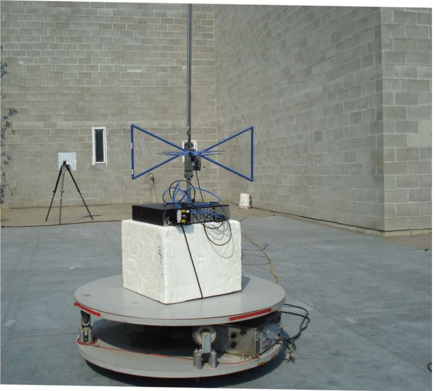
Figure E14.2 – Setup Photo – Radiated Emissions < 1GHz
