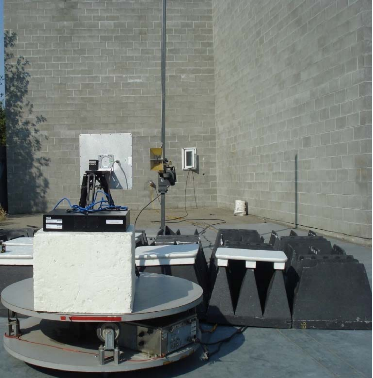
Figure E14.4 – Setup Photo – Compliance with §27.53(f) Using ZDAFP750-10-60D Antenna
