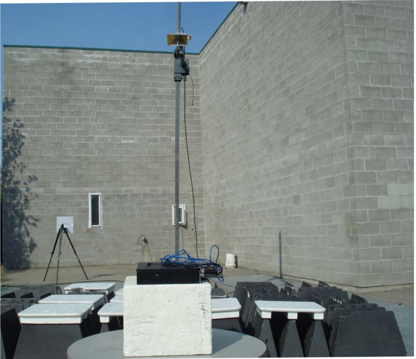
Figure E14.3 – Setup Photo – Radiated Emissions > 1GHz
