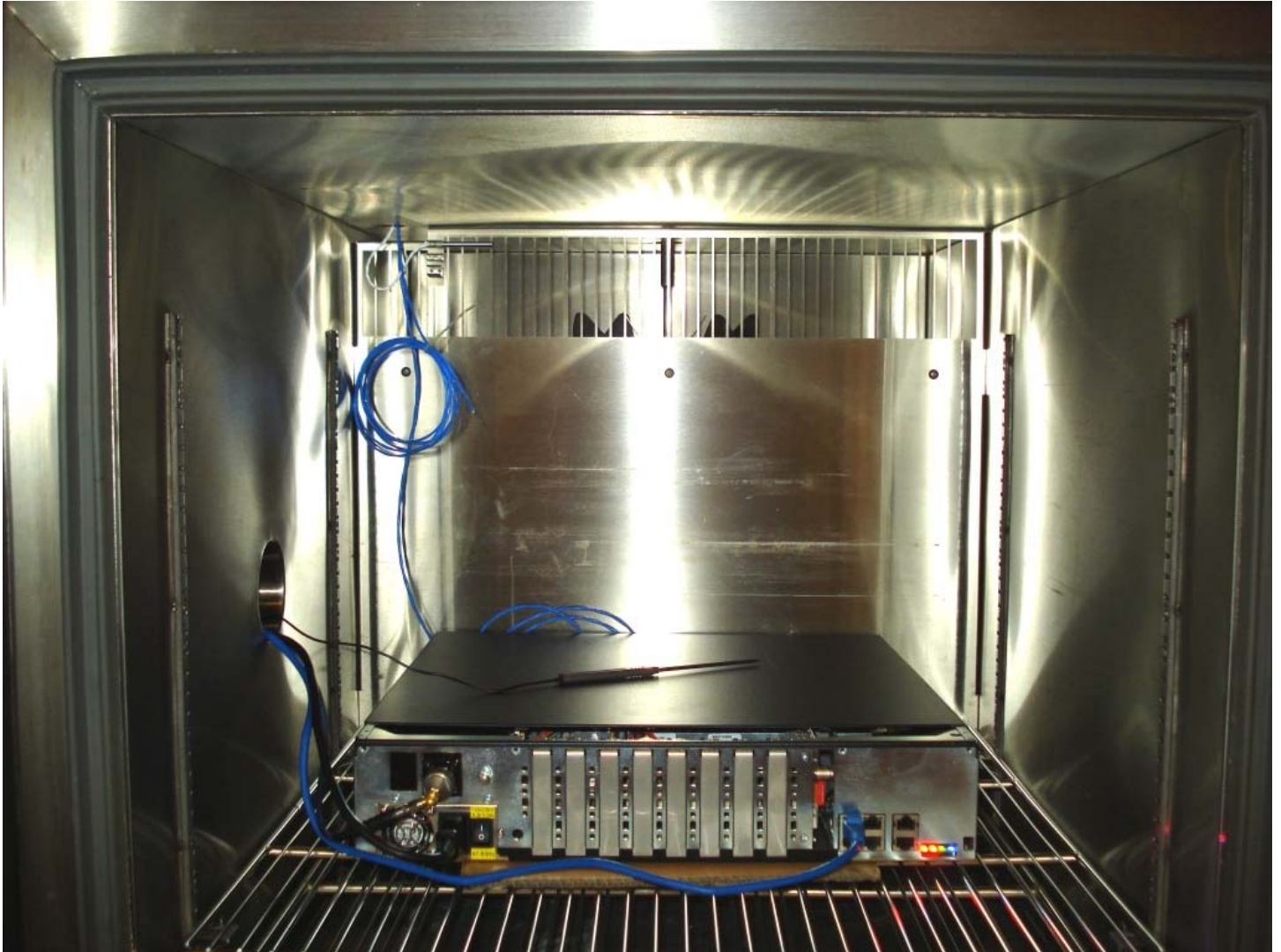
Figure E14.1 – Setup Photo – Frequency Stability in Environmental Chamber
