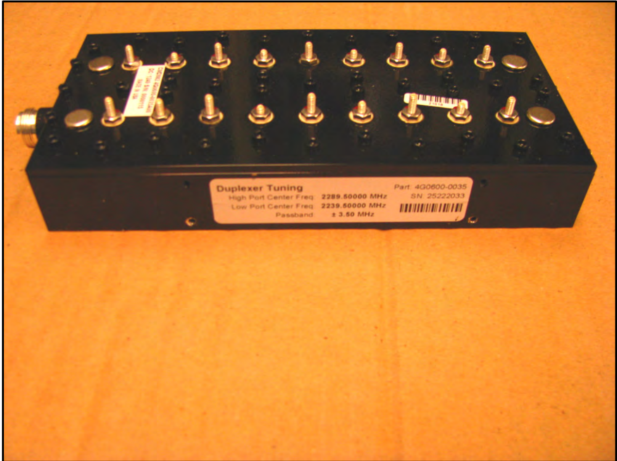
Photograph 14: Duplexer – Right Top View
