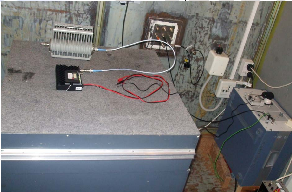
Conducted emissions setup
