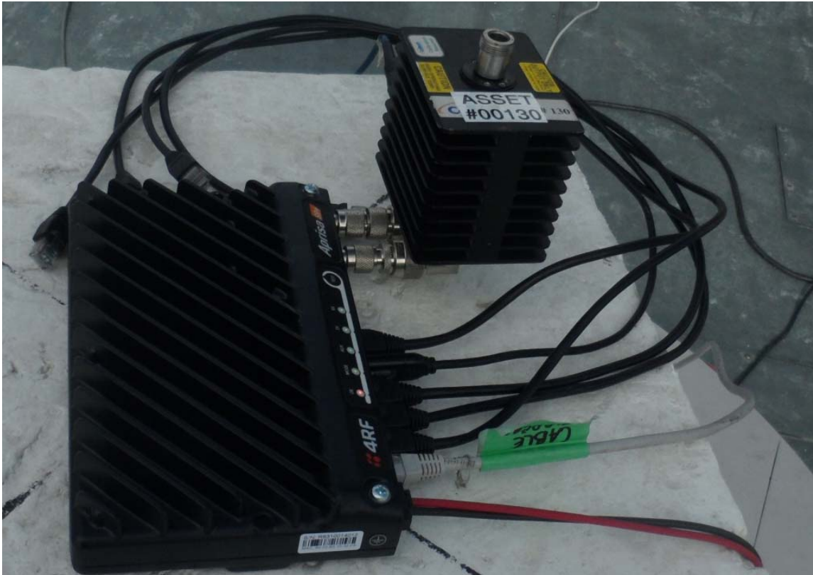
Figure E15.5 – Setup Photo – Radiated Emissions – SR+ Variant
