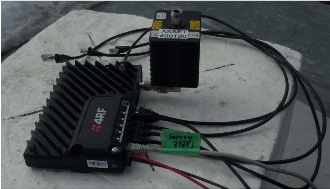
Figure E15.6 – Setup Photo – Radiated Emissions - SR Variant
