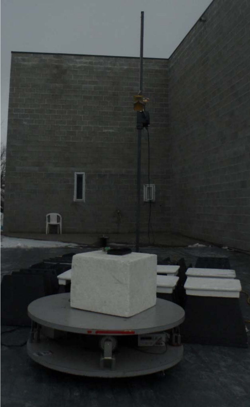
Figure E15.4 – Setup Photo – Radiated Emissions > 1GHz
