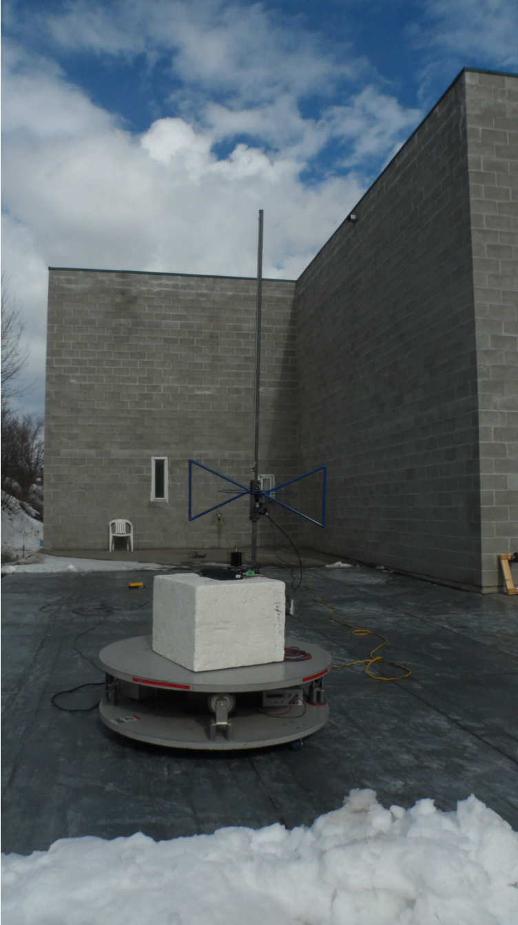
Figure E15.3 – Setup Photo – Radiated Emissions < 1GHz
