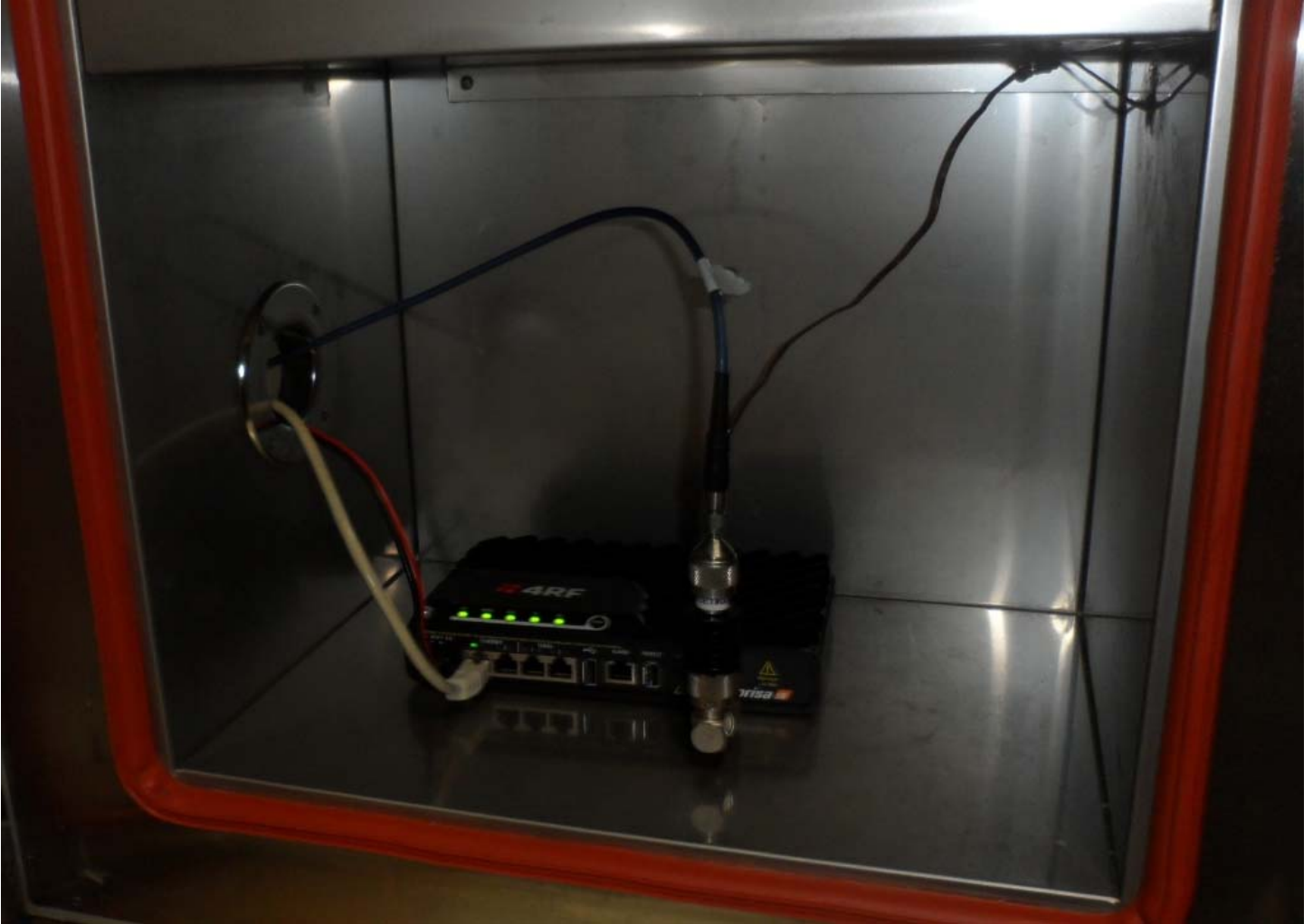
Figure E15.1 – Setup Photo – Frequency Stability in Environmental Chamber
