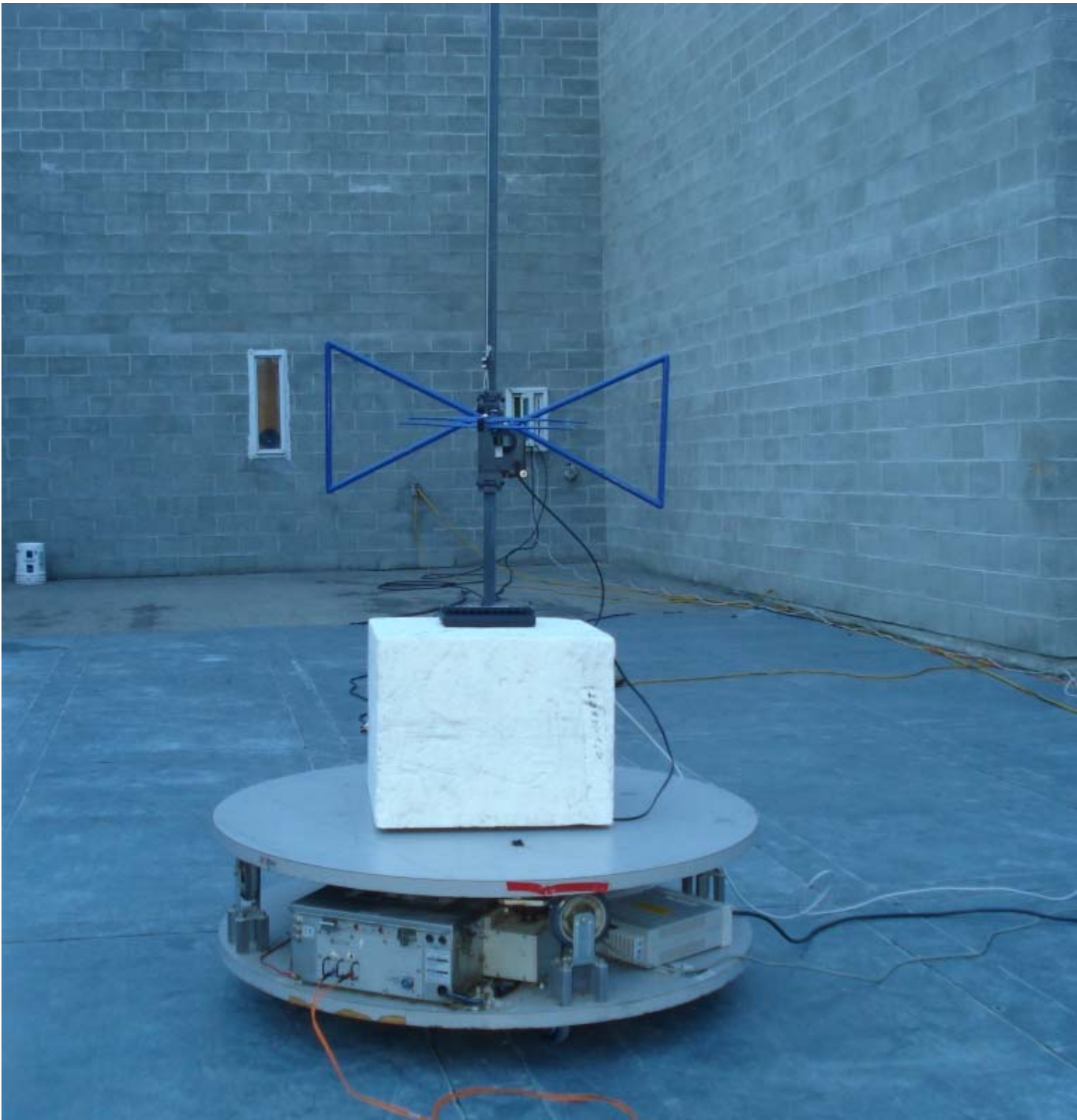
Radiated Emissions Set-Up
