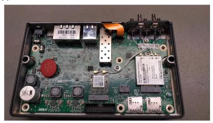
The module has three RF connectors:
