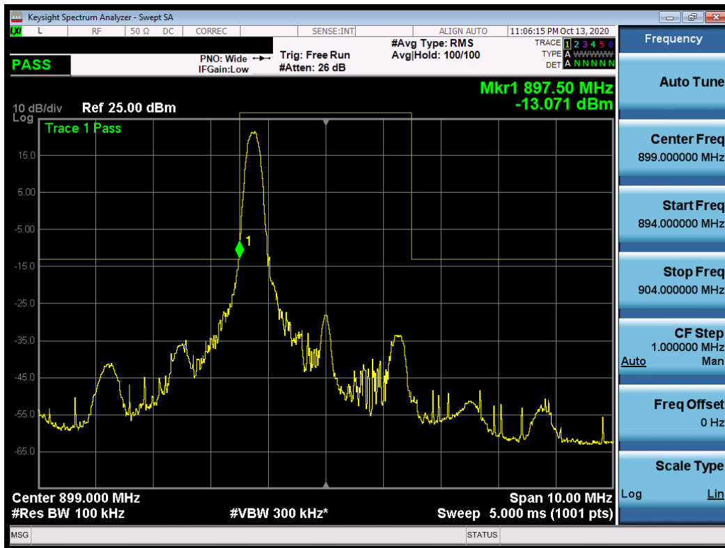
Plot 7-15. Band Edge Plot (QPSK, 1RB, RB Offset 0)
