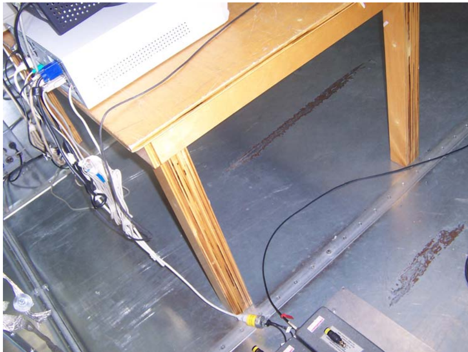
Conducted Emissions Test Setup, Rear View Showing Cable Layout
