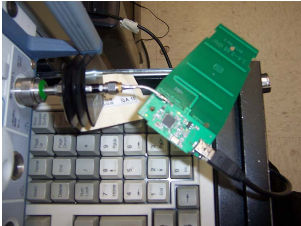
Antenna Conducted Emissions, Occupied Bandwidth, Power Output, Power Spectral Density Setup
