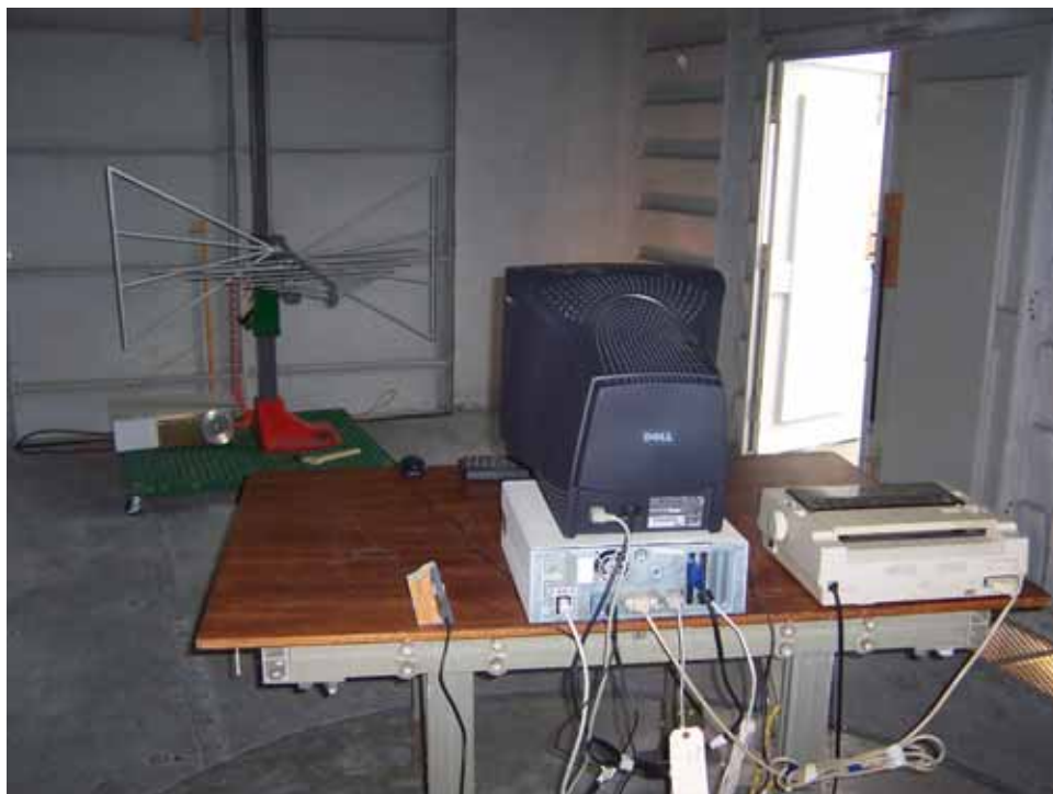
Horizontal Polarity Biconilog Antenna Test Setup
