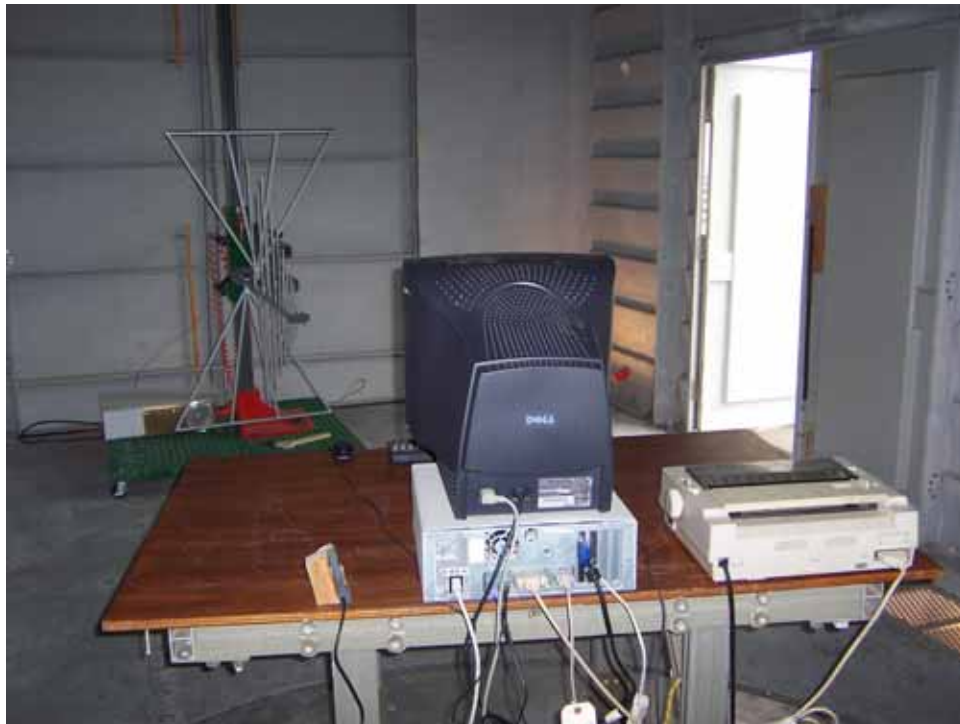
Vertical Polarity Biconilog Antenna Test Setup
