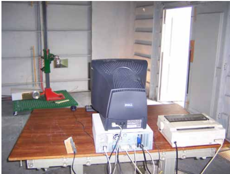
Vertical Polarity DRG Antenna Test Setup
