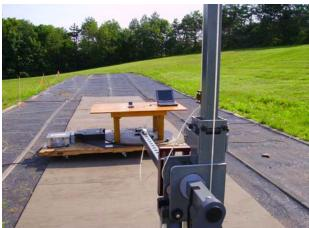
Radiated Emissions Test Setup Photographs Figure 8
