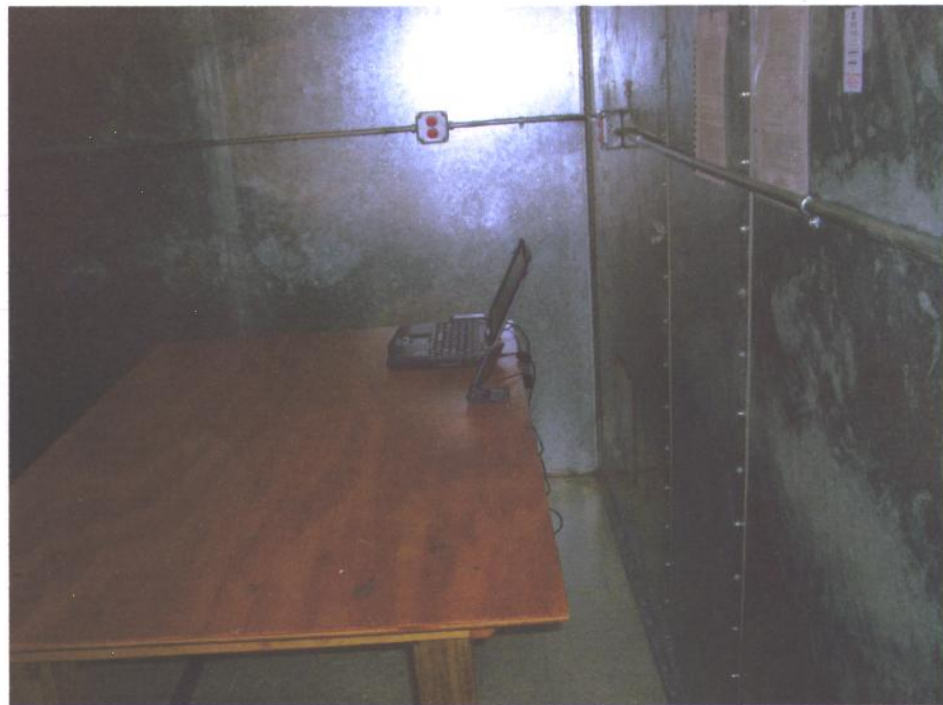
EUT 40cm from vertical ground plane
