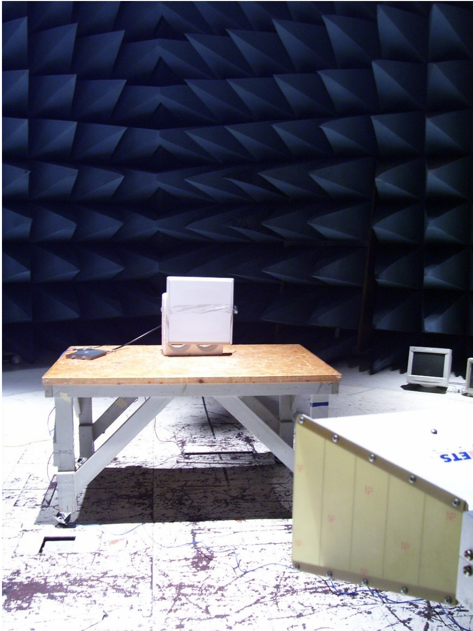
Photograph 3. Test Equipment and setup for various Radiated Measurements, 5GHz
