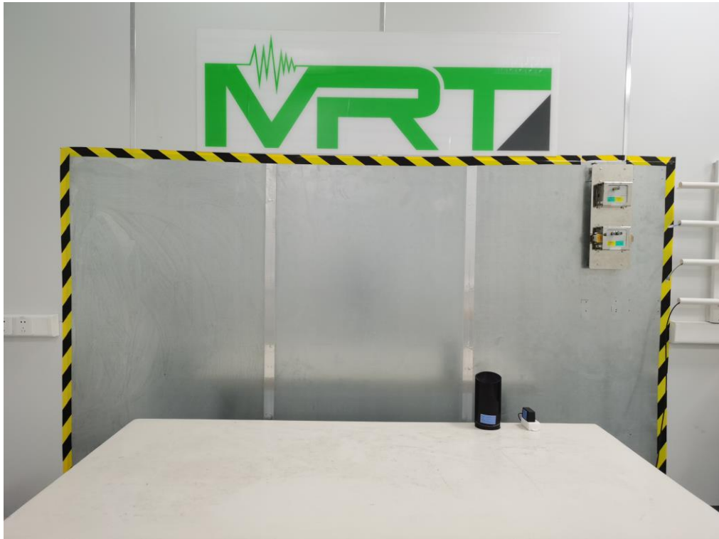
Description: Back View of Conducted Emission Test Setup for 6GHz RLAN
