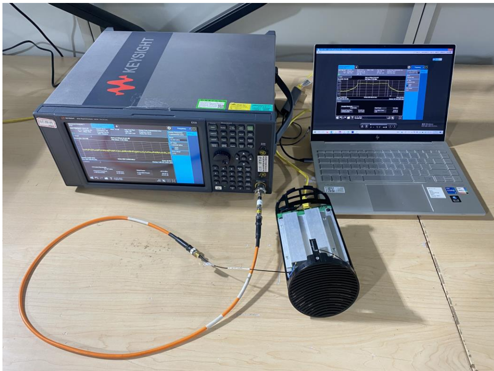
Description: 6GHz RLAN RF Conducted Test Setup
