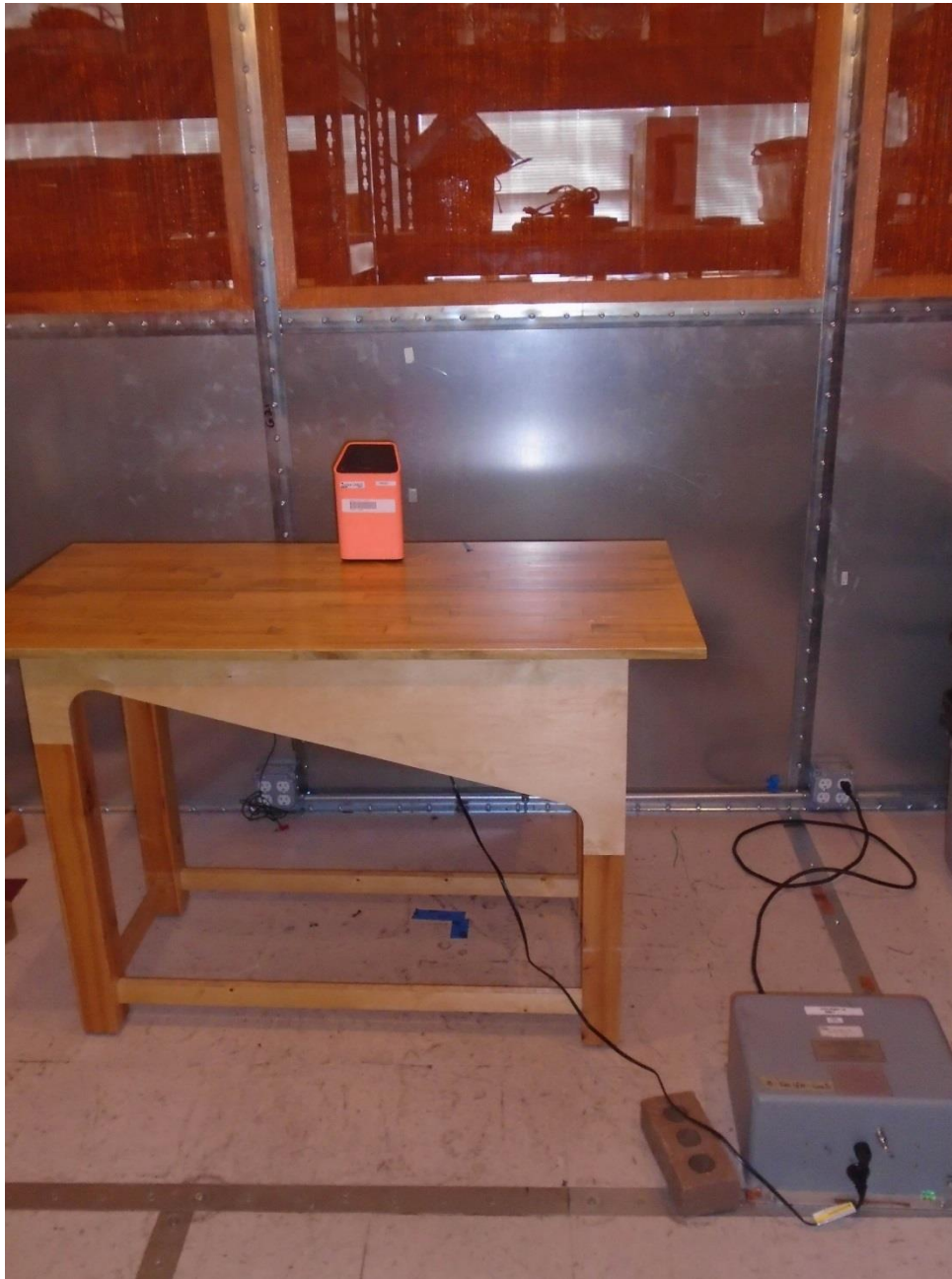
Photograph 1. Conducted Emissions, 15.207(a), Test Setup
