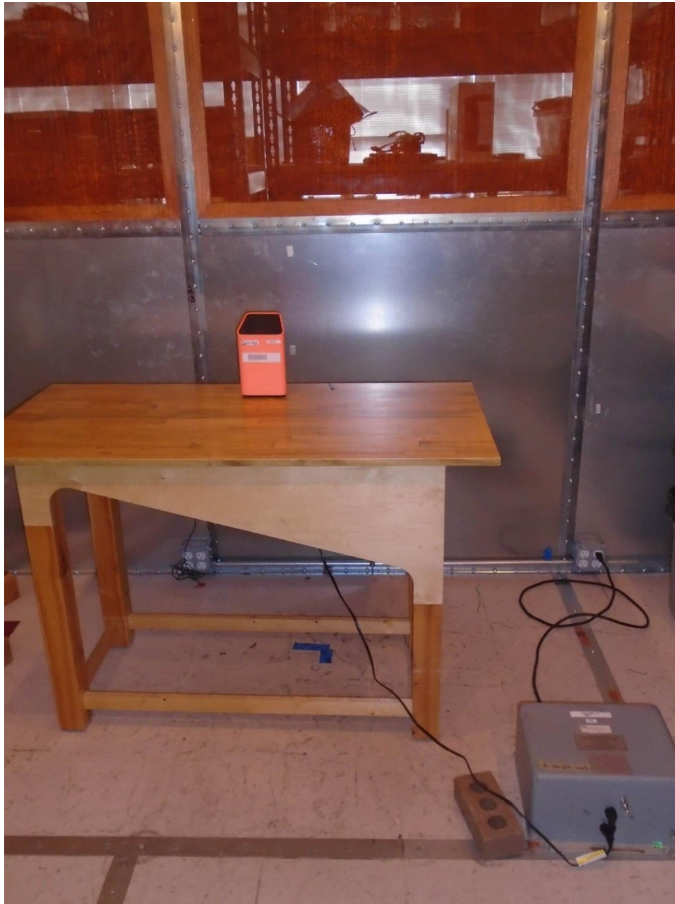
Photograph 1. Conducted Emissions, 15.207(a), Test Setup
