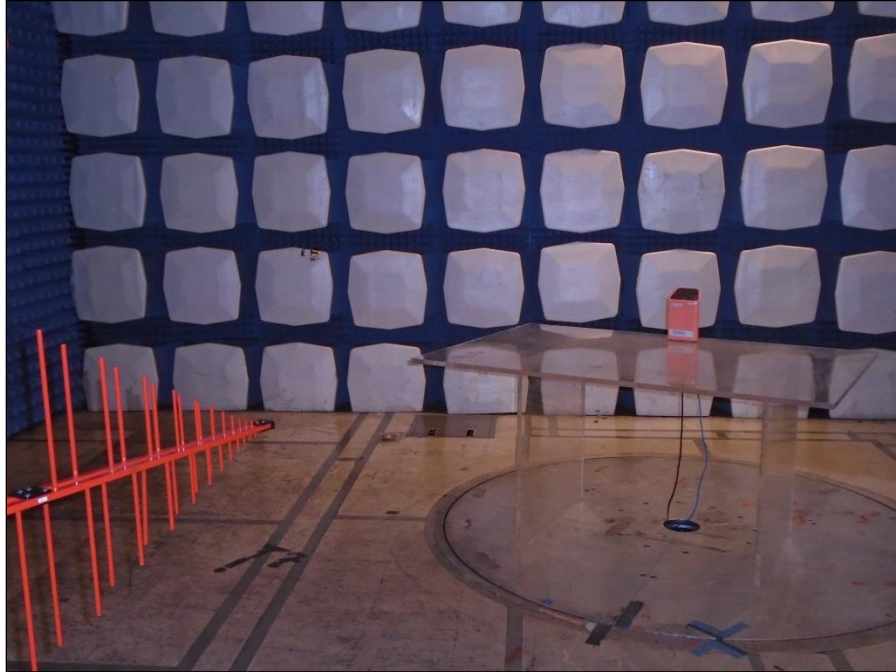
Photograph 2. Radiated Emissions, up to 1 GHz
