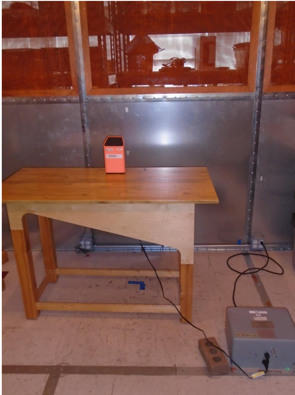
Photograph 1. Conducted Emissions, 15.207(a), Test Setup
