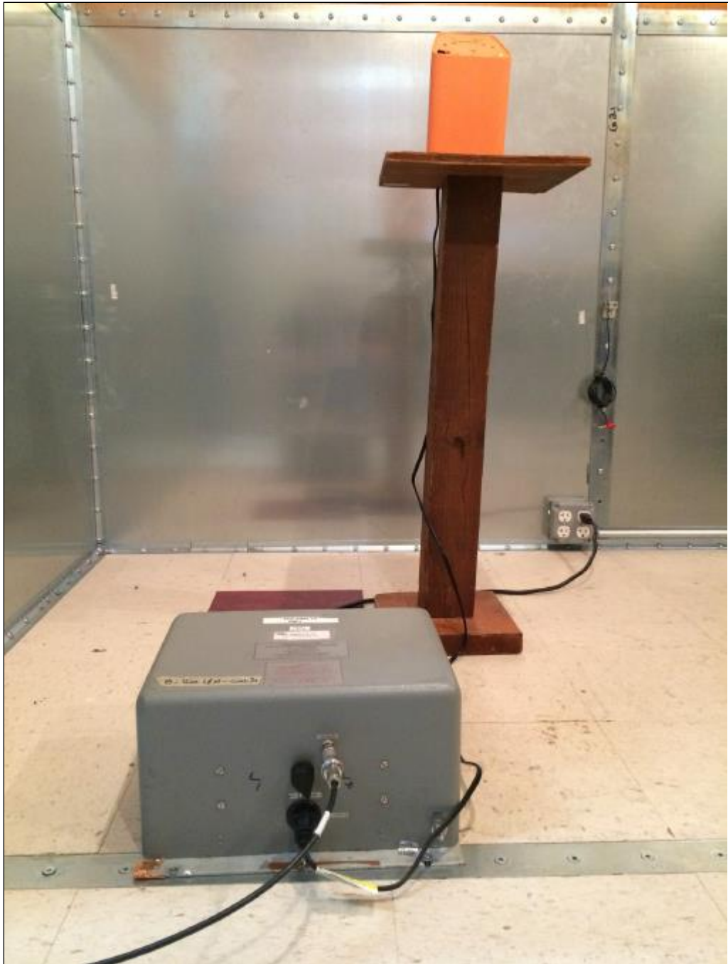
Photograph 1. Conducted Emissions, 15.207(a), Test Setup
