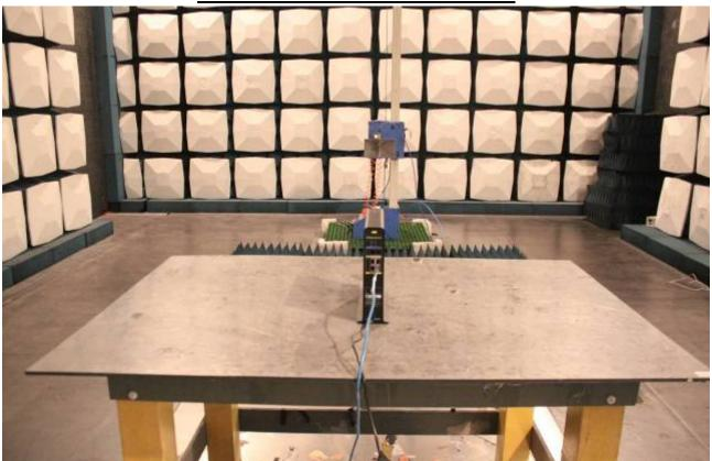
**RADIATED EMISSION TEST 30MHz to 1G**
