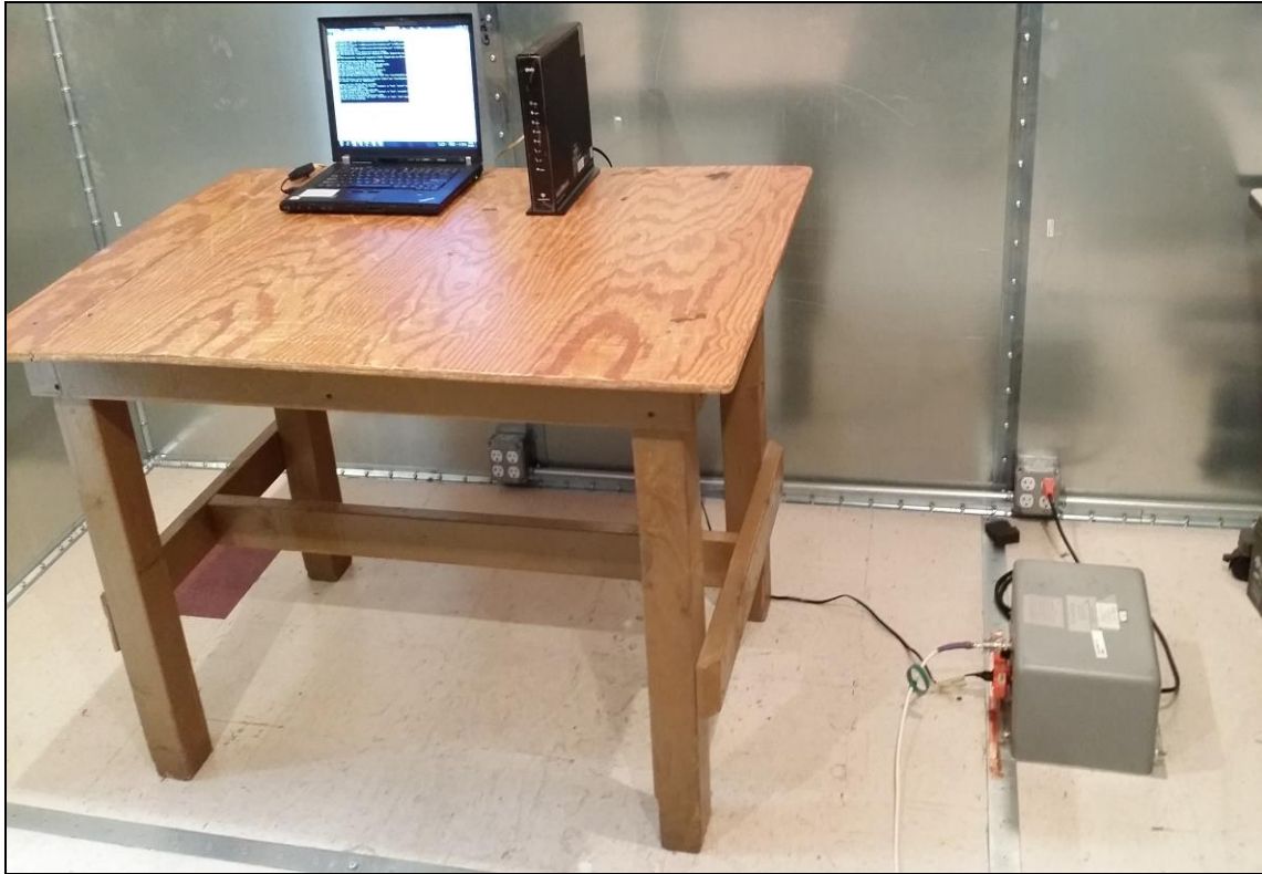
Photograph 1. Conducted Emissions, 15.207(a), Test Setup
