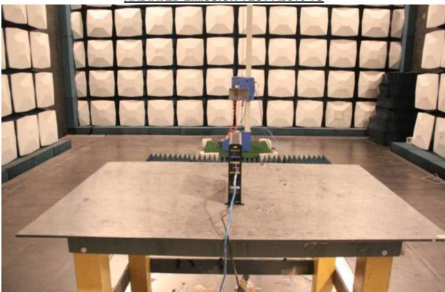
RADIATED EMISSION TEST 30MHz to 1G
