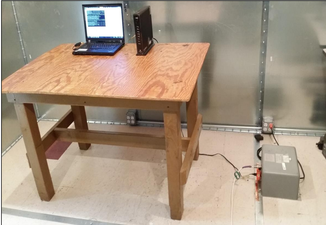
Photograph 1. Conducted Emissions, 15.207(a), Test Setup
