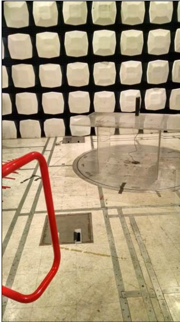
Photograph 1. Radiated Spurious Emissions, Test Setup, 30 MHz – 1 GHz
