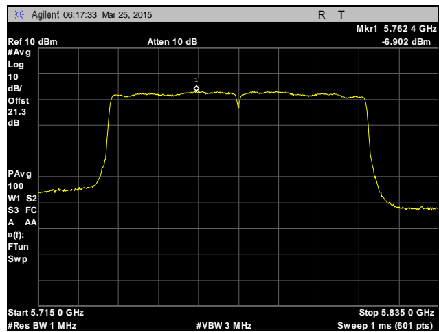
Plot 117. Peak Power Spectral Density, 802.11ac 80 MHz, MIMO, Transmitting Beam-Forming
