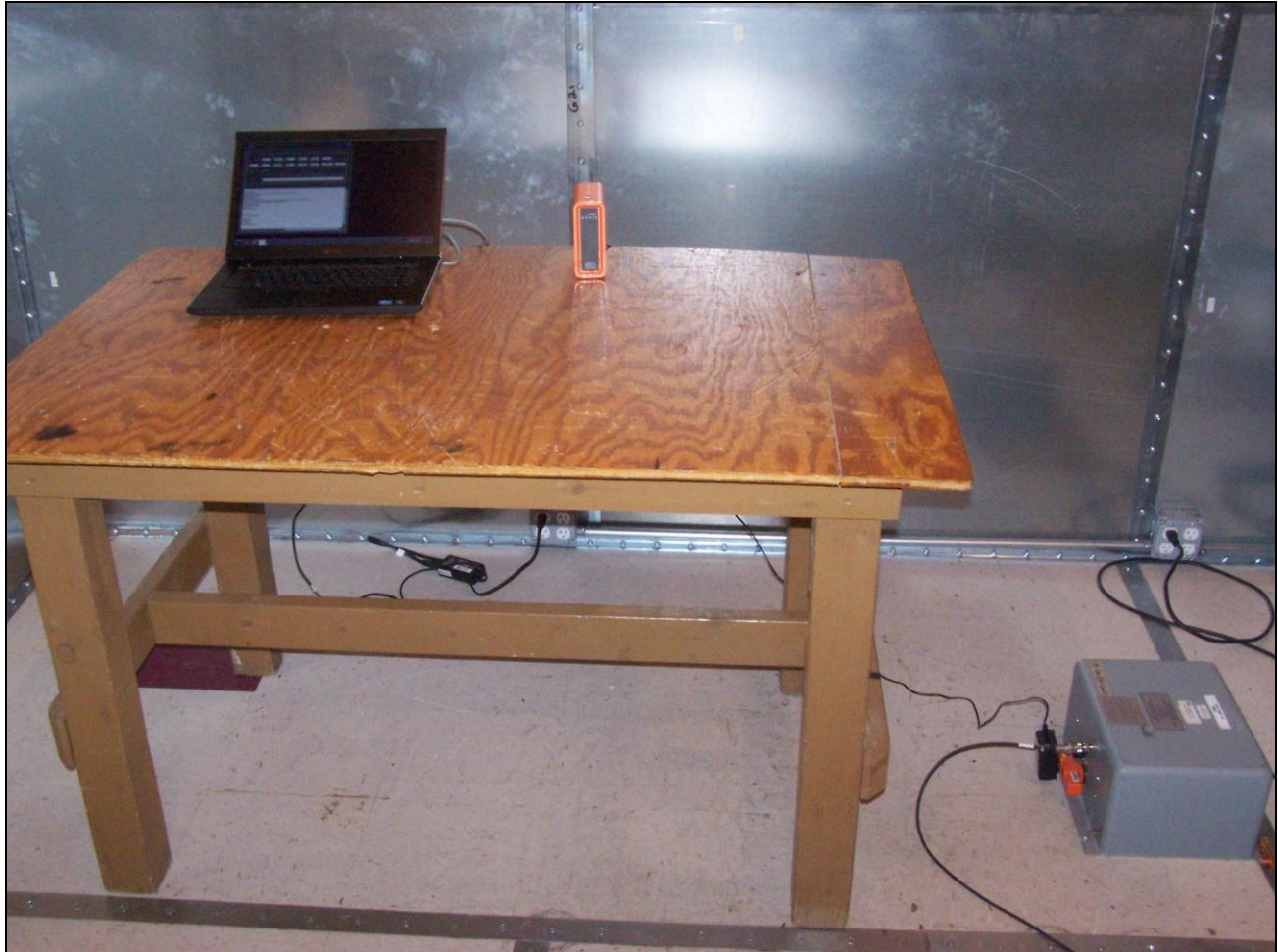
Photograph 1. Conducted Emissions, 15.207(a), Test Setup
