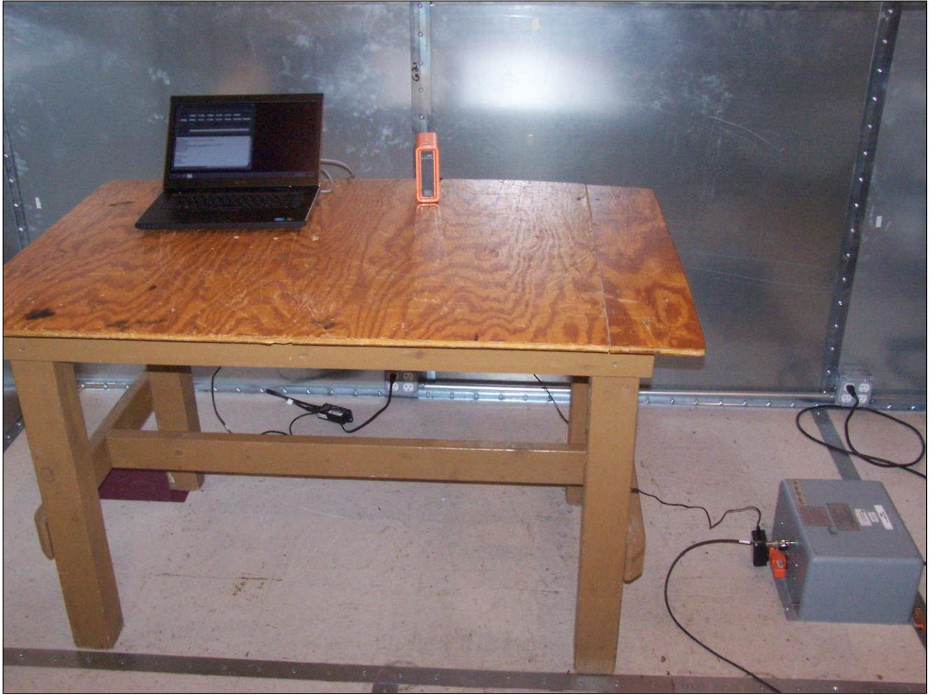
Photograph 1. Conducted Emissions, Test Setup
