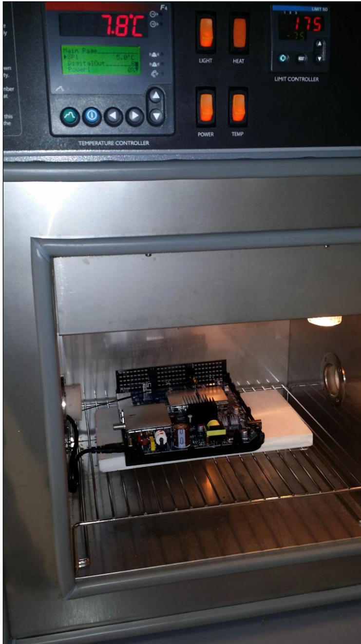
Photograph 6. Frequency Stability, Test Setup
