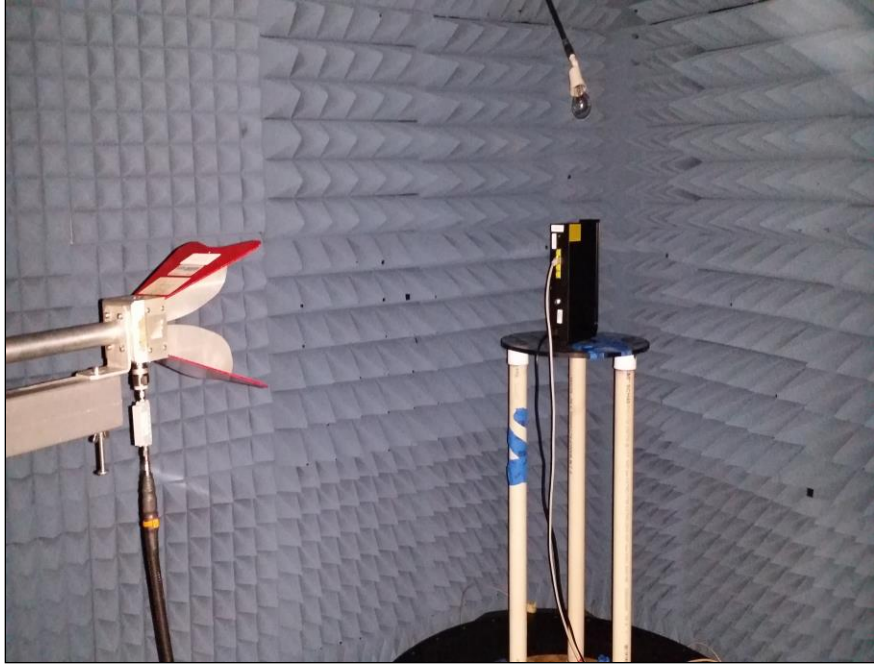
Photograph 5. Radiated Spurious Emissions, Test Setup, Above 1 GHz
