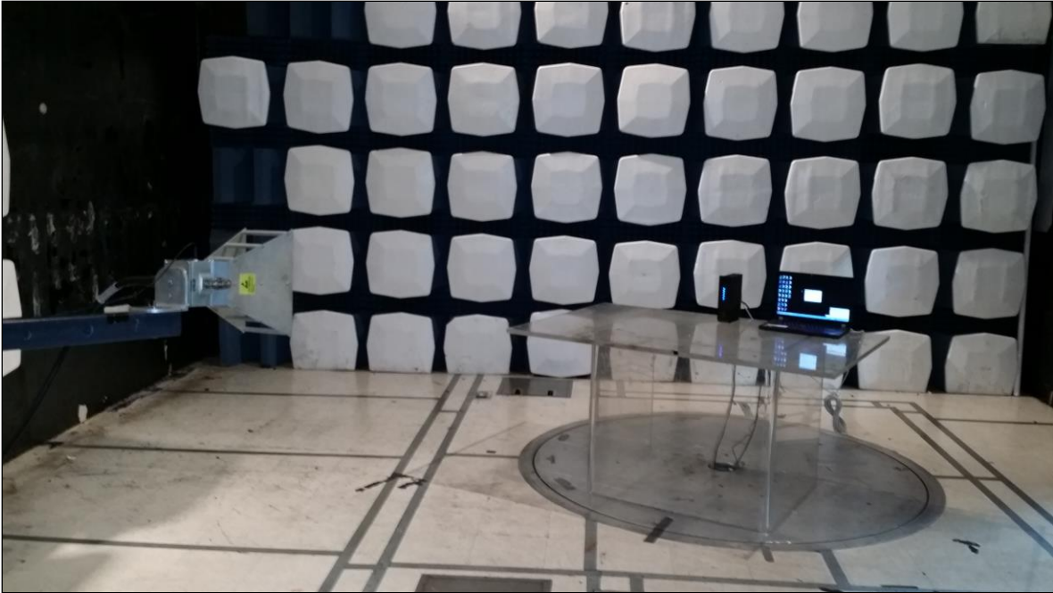
Photograph 3. Radiated Emission, Test Setup, Above 1 GHz
