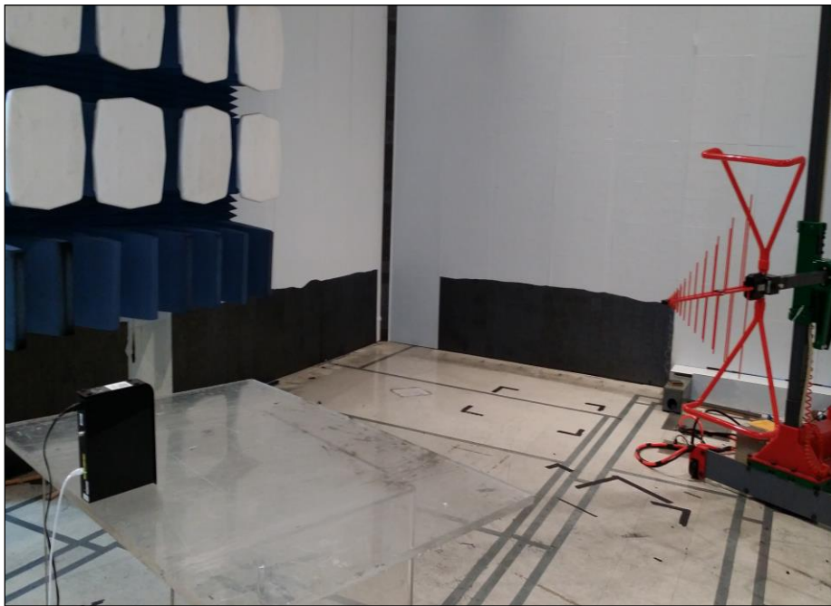
Photograph 4. Radiated Spurious Emissions, Test Setup, 30 MHz – 1 GHz
