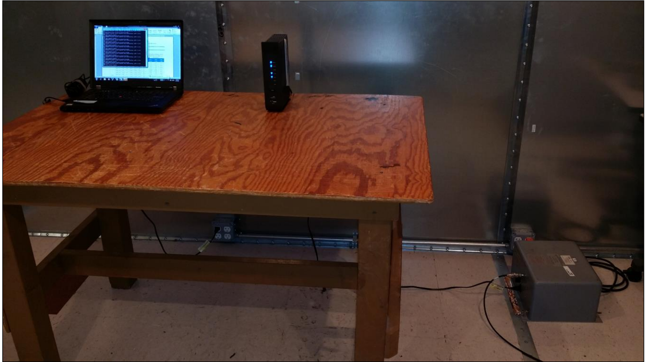
Photograph 1. Conducted Emissions, 15.207(a), Test Setup
