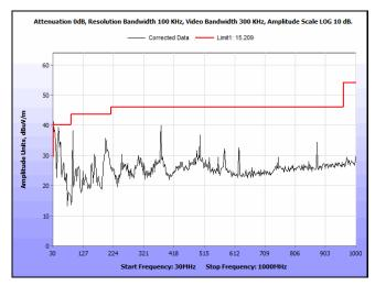
Plot 85. Radiated Spurious Emissions, 5200 MHz, 802.11a, 30 MHz - 1 GHz
