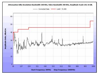
Plot 103. Radiated Spurious Emissions, 5200 MHz, 802.11n, HT40, 30 MHz - 1 GHz
