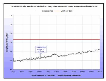
Plot 90. Radiated Spurious Emissions, 5240 MHz, 802.11a, 7 GHz - 18 GHz
