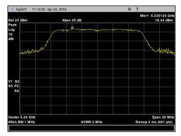
Plot 71. Peak Power Spectral Density, 5240 MHz, 802.11n, HT20, Chain 1
