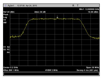
Plot 69. Peak Power Spectral Density, 5200 MHz, 802.11n, HT20, Chain 2
