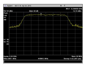
Plot 70. Peak Power Spectral Density, 5240 MHz, 802.11n, HT20, Chain 0
