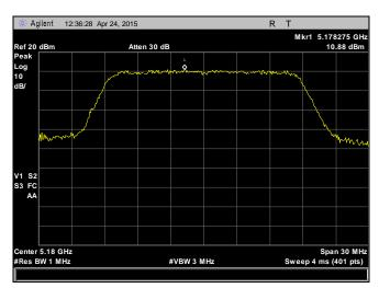
Plot 66. Peak Power Spectral Density, 5180 MHz, 802.11n, HT20, Chain 2
