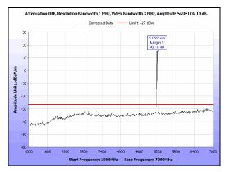
Plot 83. Radiated Spurious Emissions, 5180 MHz, 802.11a, 1 GHz - 7 GHz
