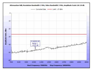
Plot 99. Radiated Spurious Emissions, 5240 MHz, 802.11n, HT20, 7 GHz – 18 GHz
