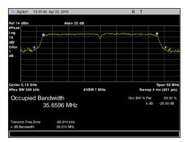
Plot 21. 26 dB Occupied Bandwidth, 5190 MHz, 802.11n, HT40, Chain 2
