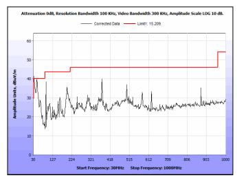
Plot 88. Radiated Spurious Emissions, 5240 MHz, 802.11a, 30 MHz - 1 GHz
