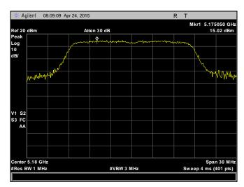
Plot 58. Peak Power Spectral Density, 5200 MHz, 802.11a, Chain 0
