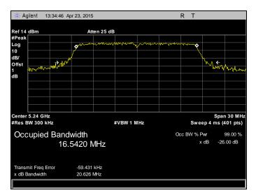
Plot 9. 26 dB Occupied Bandwidth, 5240 MHz, 802.11a, Chain 2
