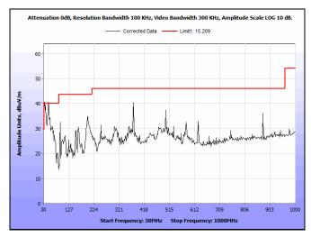
Plot 100. Radiated Spurious Emissions, 5190 MHz, 802.11n, HT40, 30 MHz - 1 GHz
