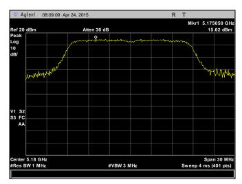
Plot 64. Peak Power Spectral Density, 5180 MHz, 802.11n, HT20, Chain 0
