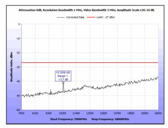
Plot 93. Radiated Spurious Emissions, 5180 MHz, 802.11n, HT20, 7 GHz – 18 GHz
