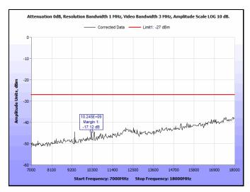
Plot 102. Radiated Spurious Emissions, 5190 MHz, 802.11n, HT40, 7 GHz – 18 GHz
