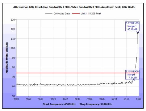
Plot 110. Radiated Band Edge, 5180 MHz, Peak, 802.11a
