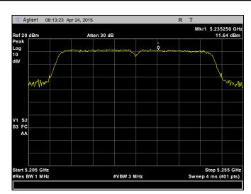
Plot 79. Peak Power Spectral Density, 5230 MHz, 802.11n, HT40, Chain 0
