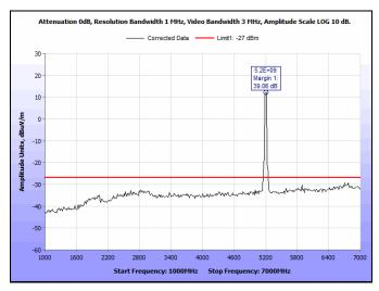
Plot 104. Radiated Spurious Emissions, 5200 MHz, 802.11n, HT40, 1 GHz – 7 GHz
