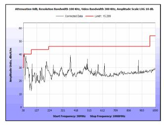
Plot 94. Radiated Spurious Emissions, 5200 MHz, 802.11n, HT20, 30 MHz - 1 GHz
