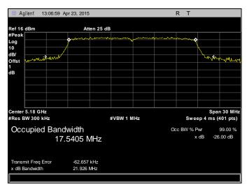
Plot 11. 26 dB Occupied Bandwidth, 5180 MHz, 802.11n, HT20, Chain 1
