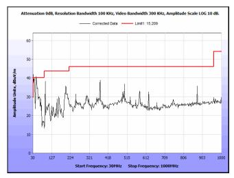
Plot 91. Radiated Spurious Emissions, 5180 MHz, 802.11n, HT20, 30 MHz - 1 GHz
