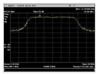
Plot 57. Peak Power Spectral Density, 5180 MHz, 802.11a, Chain 2
