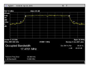
Plot 12. 26 dB Occupied Bandwidth, 5180 MHz, 802.11n, HT20, Chain 2
