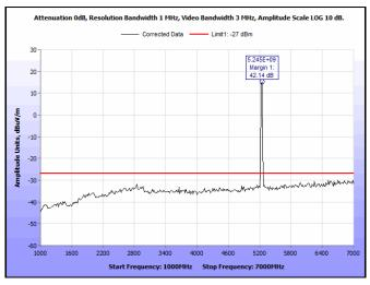
Plot 89. Radiated Spurious Emissions, 5240 MHz, 802.11a, 1 GHz - 7 GHz
