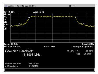
Plot 6. 26 dB Occupied Bandwidth, 5200 MHz, 802.11a, Chain 2
