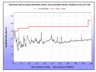
Plot 82. Radiated Spurious Emissions, 5180 MHz, 802.11a, 30 MHz - 1 GHz
