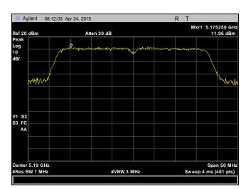
Plot 73. Peak Power Spectral Density, 5190 MHz, 802.11n, HT40, Chain 0
