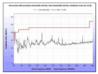
Plot 106. Radiated Spurious Emissions, 5230 MHz, 802.11n, HT40, 30 MHz - 1 GHz
