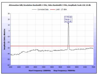
Plot 101. Radiated Spurious Emissions, 5190 MHz, 802.11n, HT40, 1 GHz - 7 GHz
