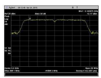
Plot 76. Peak Power Spectral Density, 5200 MHz, 802.11n, HT40, Chain 0
