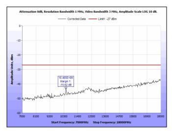
Plot 108. Radiated Spurious Emissions, 5230 MHz, 802.11n, HT40, 7 GHz – 18 GHz
