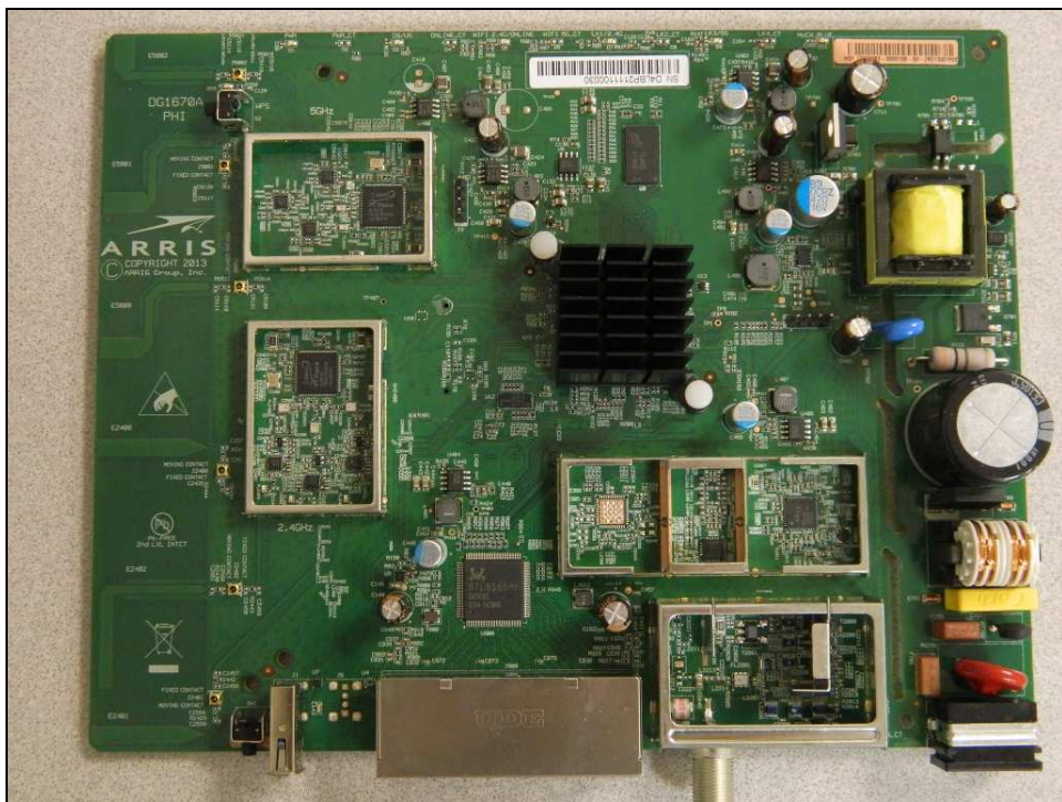
Figure 4: Internal Photo – DG1660A – Shields Removed
