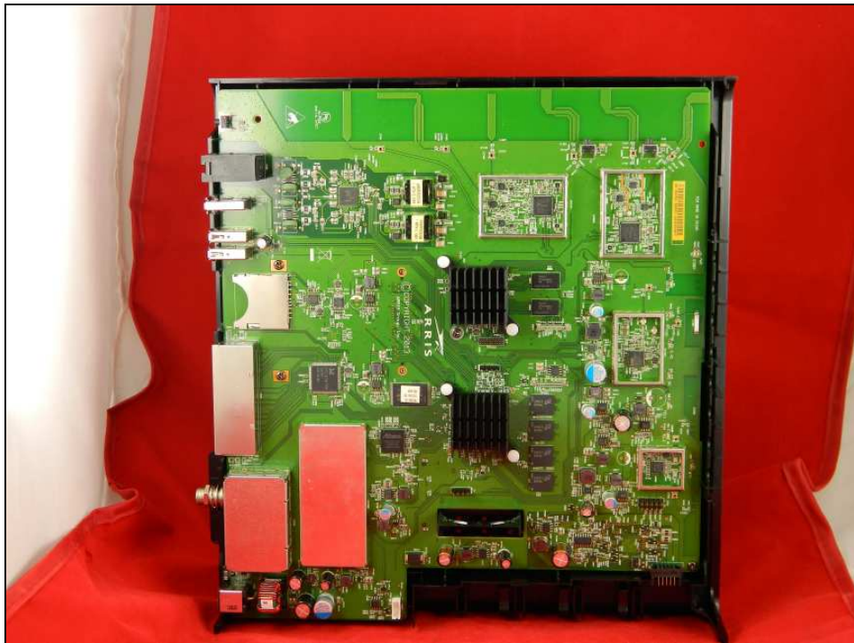
Figure 5: Internal Photo (Shields Removed)
