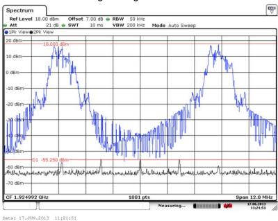
6.11.7.6 Plot demonstrating when Ch 4 is lower then Ch 2, EUT Transmits on Ch 4
