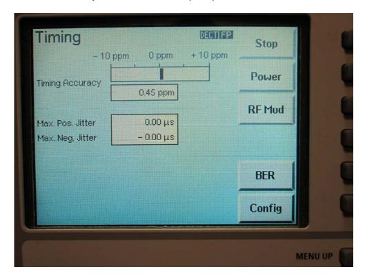
**Note:** The tester is configured for 1000 bursts of analysis (its maximum) and then monitored for a minimum of 1000 seconds recording the maximum and minimum values of jitter to satisfy the measurement requirement over 100,000 frames.
