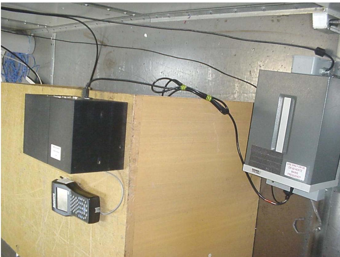
**Radiated Emissions Test Setup (EUT in transmit mode)**
