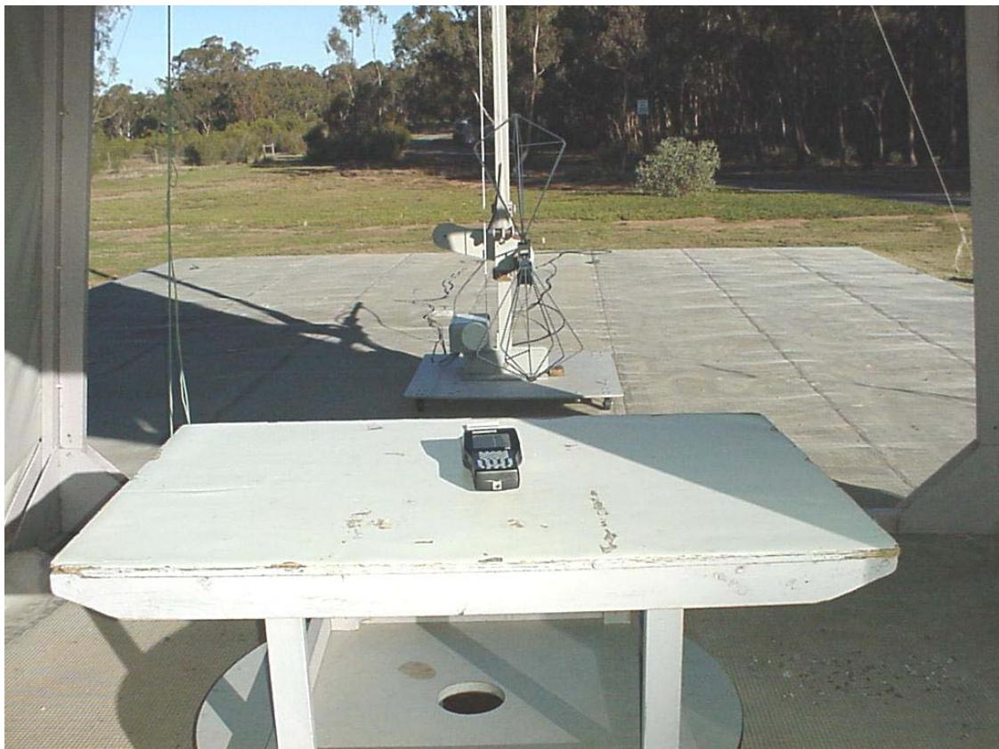
**Peak Output Power, Bandedge and Bandwidth Test Setup**
