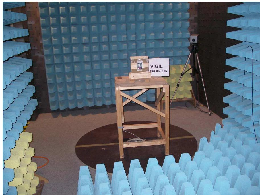
**Test setup for radiated emission measurement
