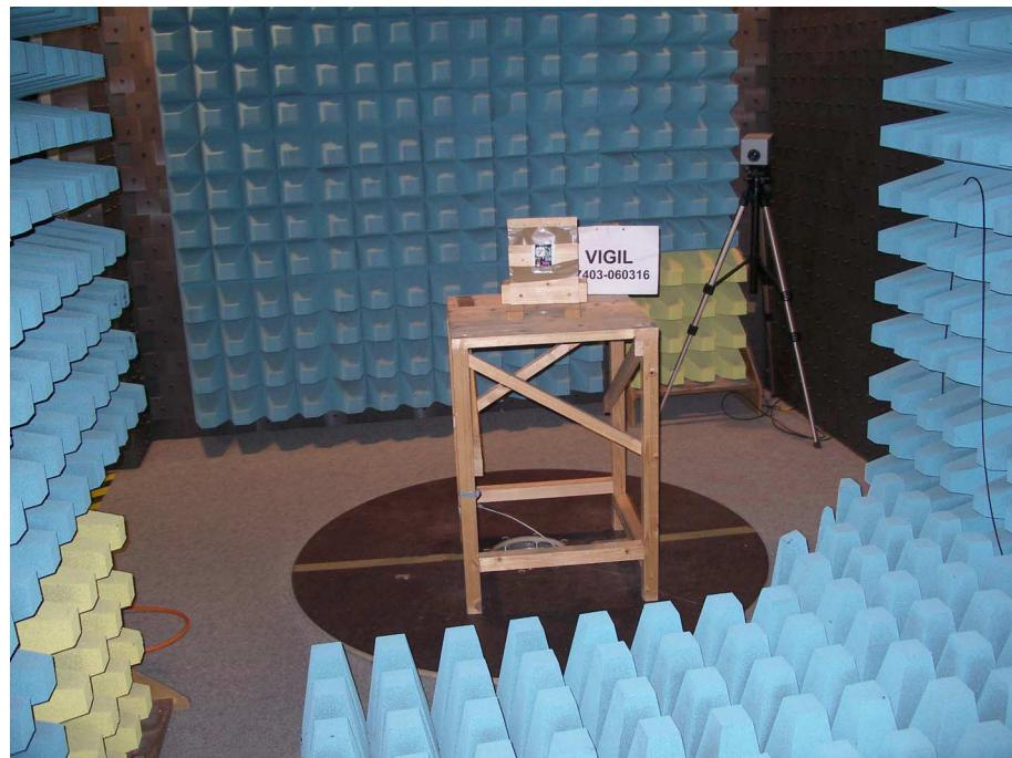
**Test setup for radiated emission measurement
