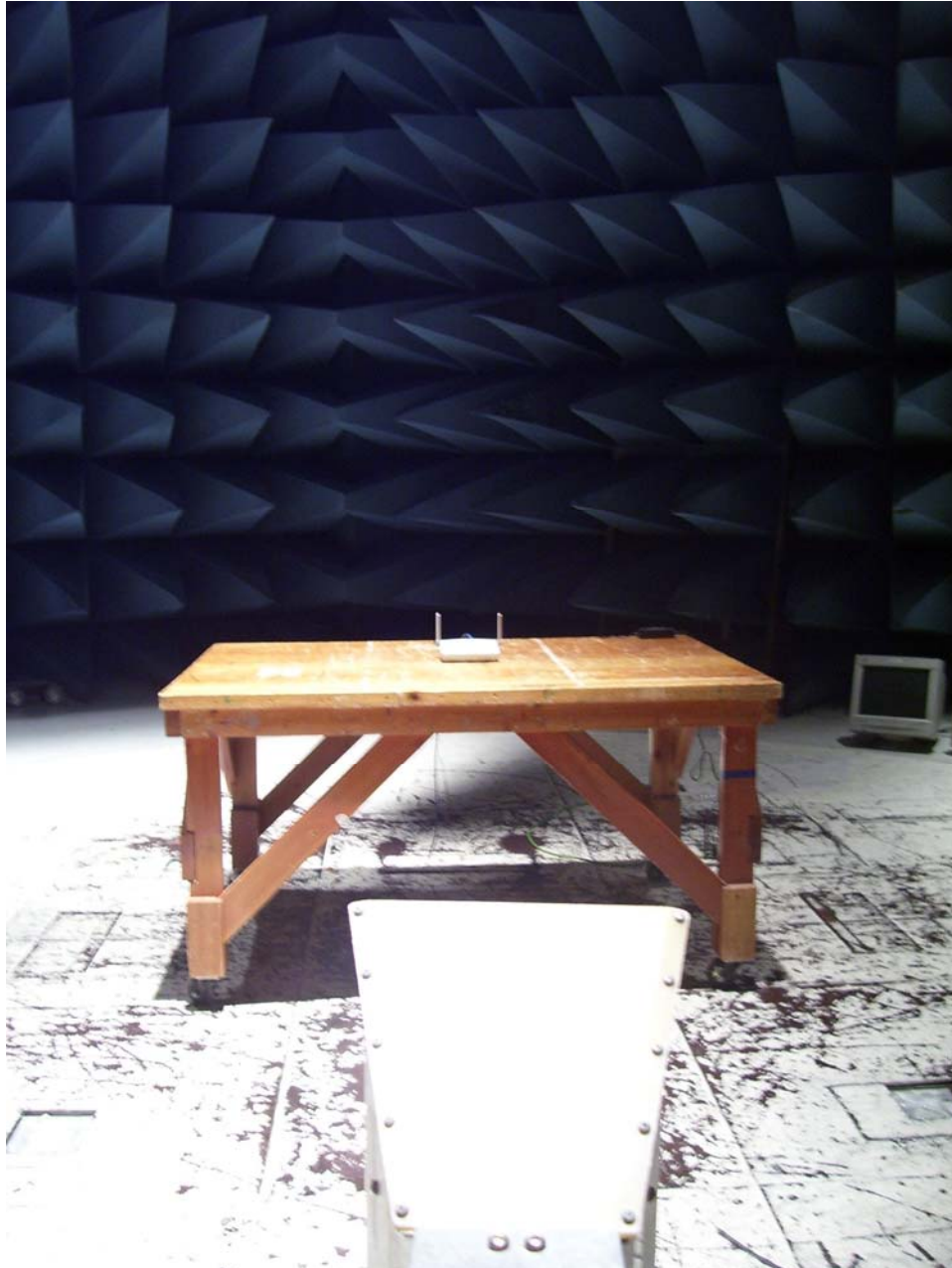
Photograph 4. Radiated Emission Test Setup
