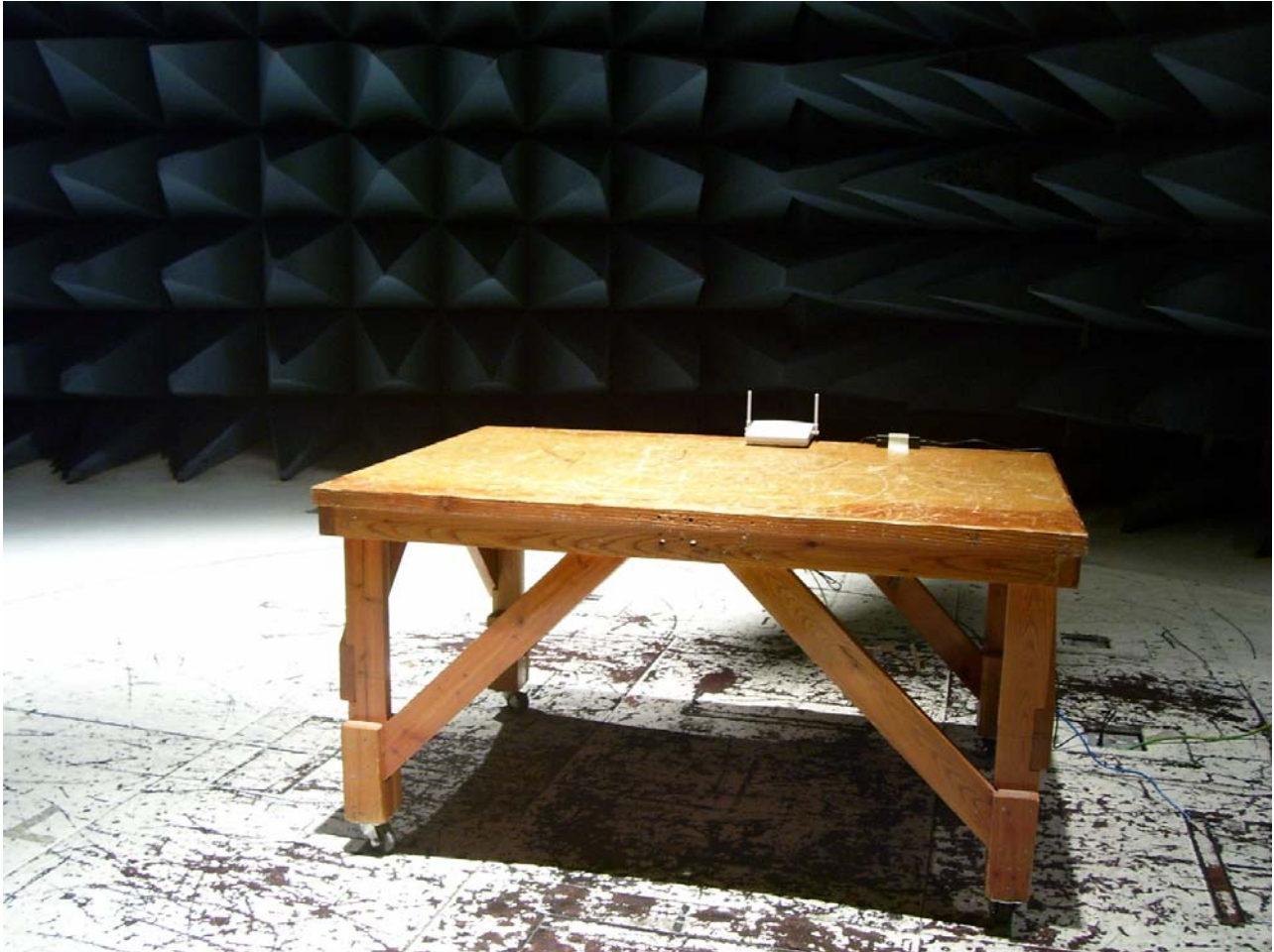
Photograph 3. Radiated Emission Test Setup 30 MHz - 1 GHz
