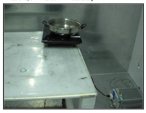
Radiated Emissions, 9 kHz to 30 MHz Test Setup
