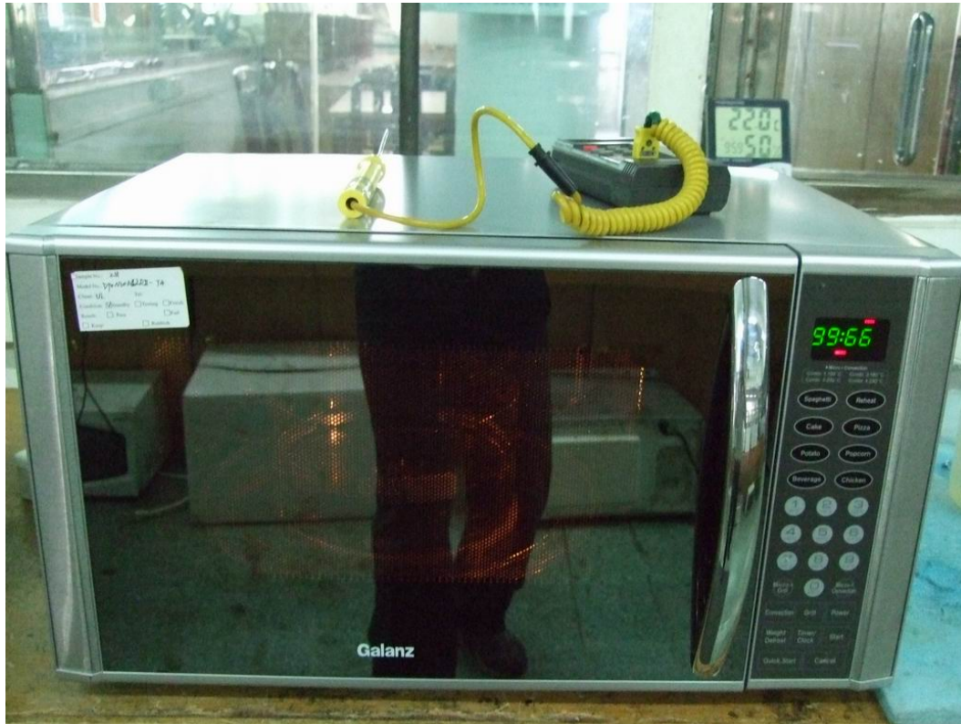
RF Output Power Test Set-up
