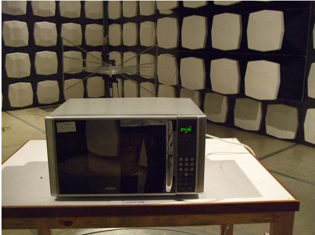
Radiated Emission Test Set-up(30-1000MHz)
