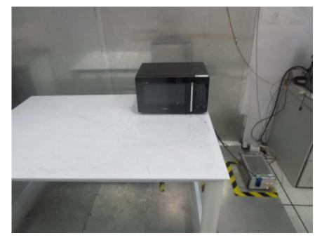
1.2 Radiated Emissions (30MHz-1GHz) Test Setup
