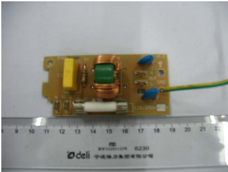
AC power filter board
