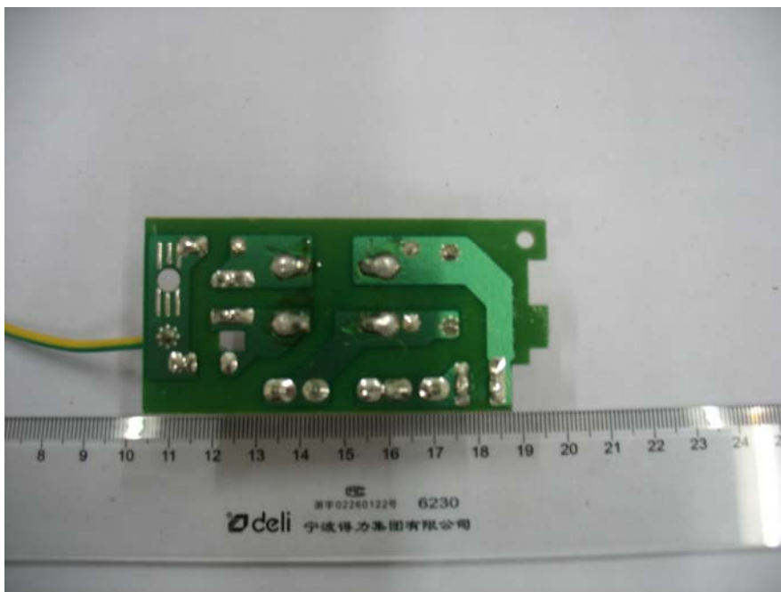
AC power filter board - Reversed
