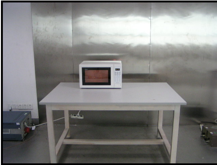
Conducted Emission - Front View
