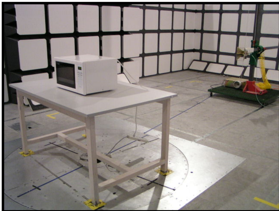
1 GHz-25GHz: Radiated Emission - Front View
