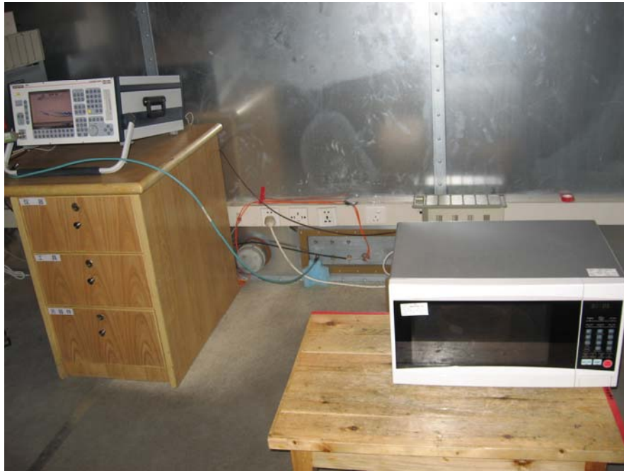
Conducted Emission Test Set-up
