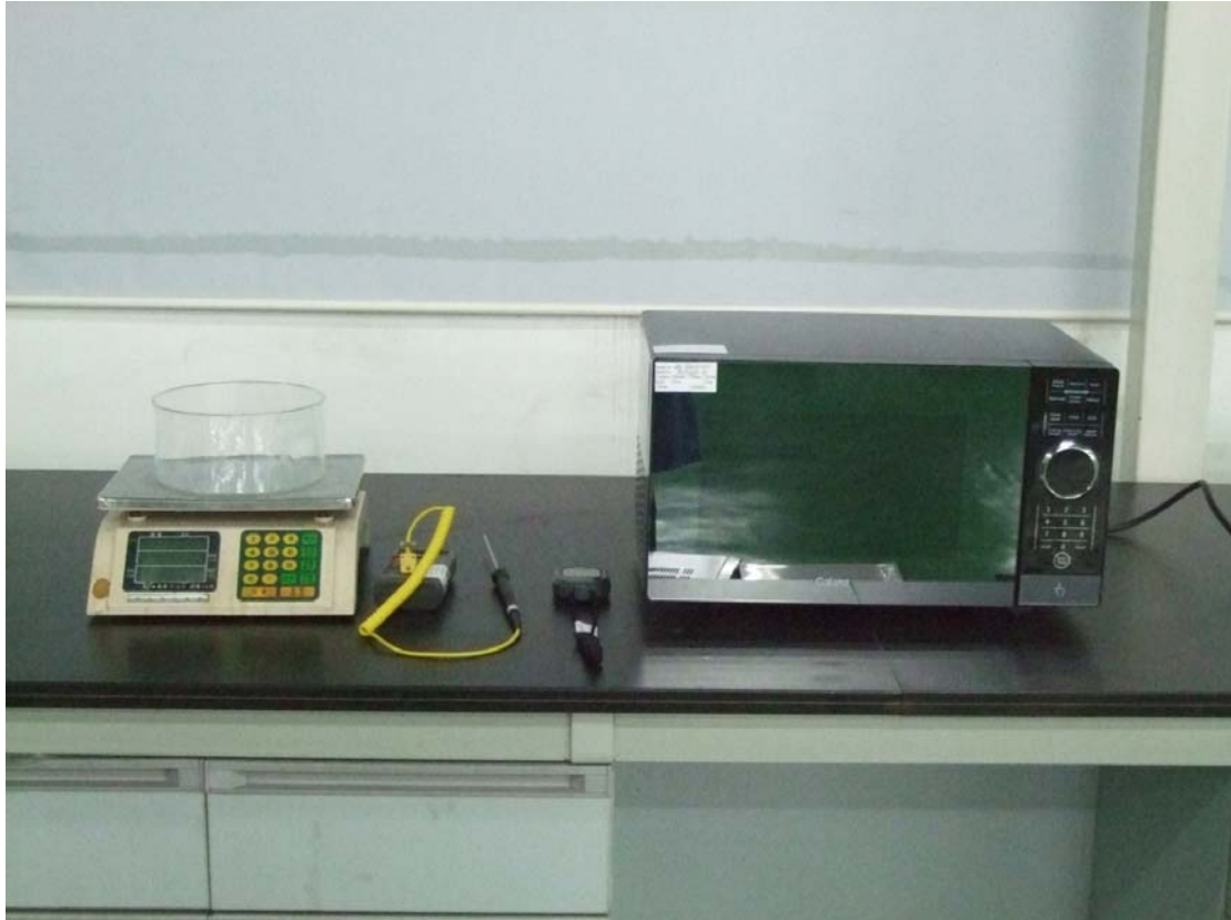
RF Output Power Test Set-up
