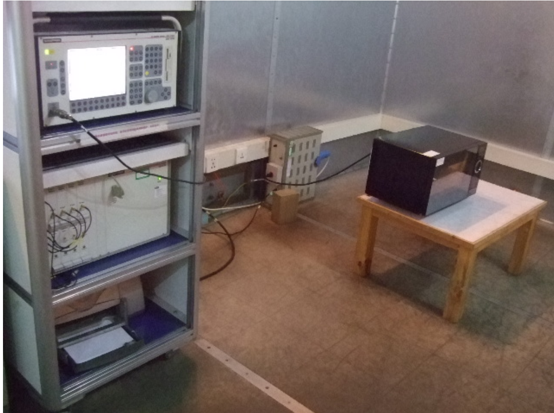
Conducted Emission Test Set-up
