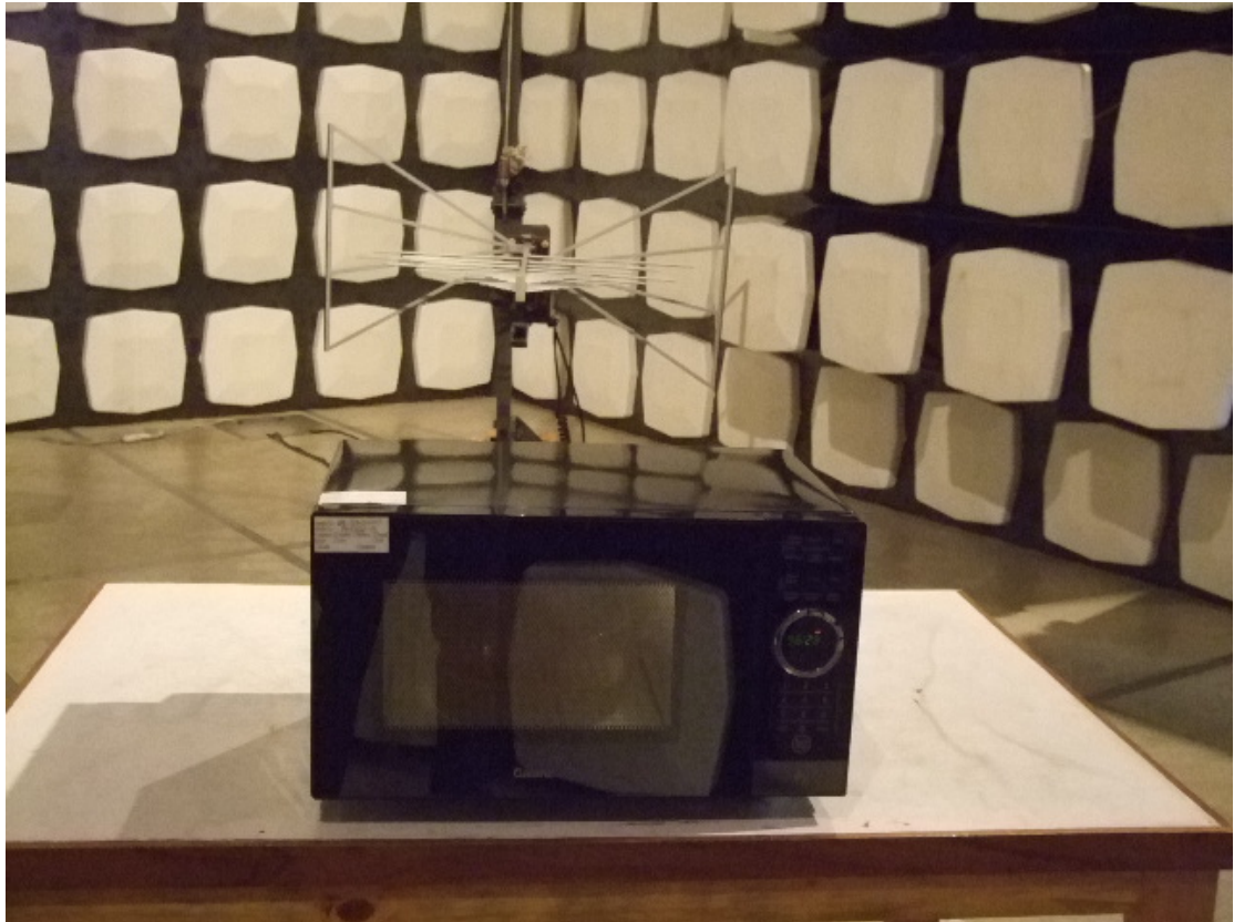
Radiated Emission Test Setup (30-1000MHz)
