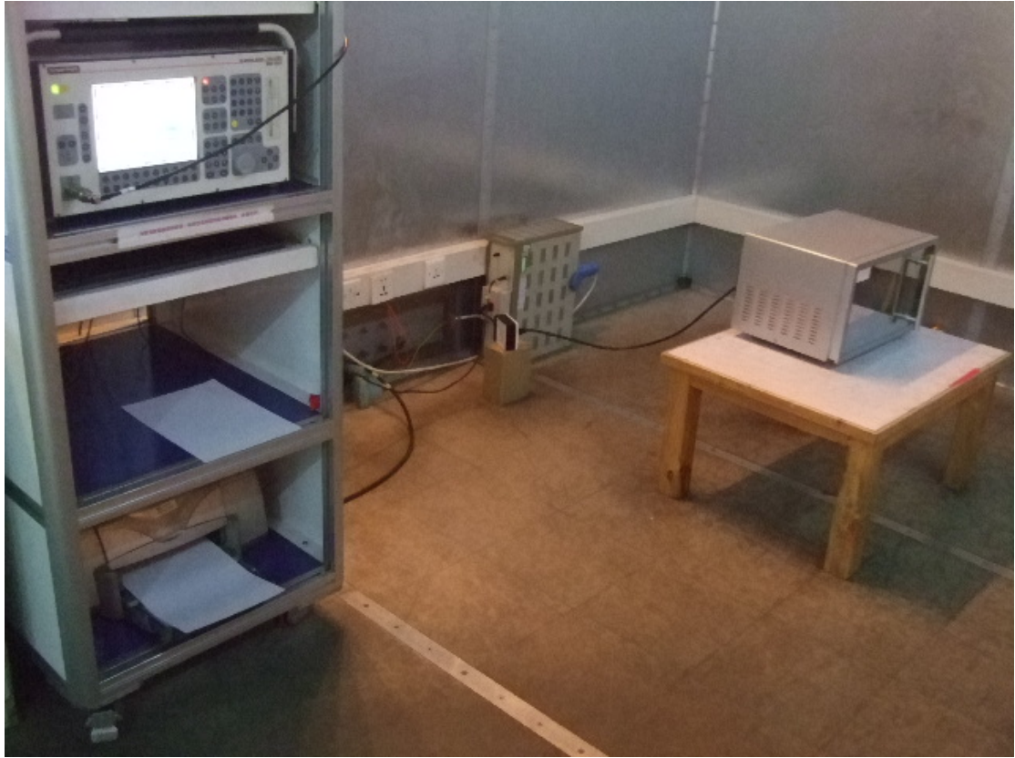
Conducted Emission Test Set-up
