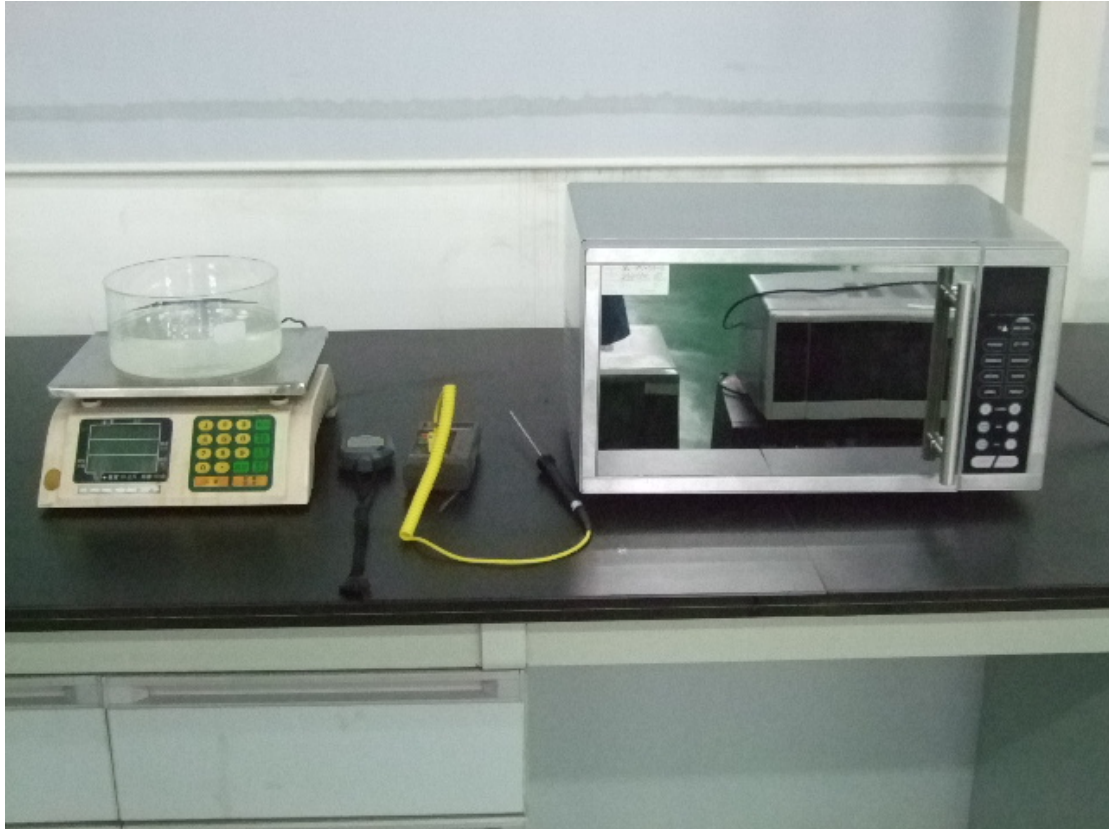
RF Output Power Test Set-up
