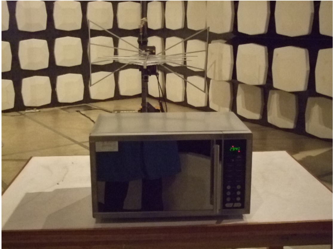
Radiated Emission Test Setup (30-1000MHz)
