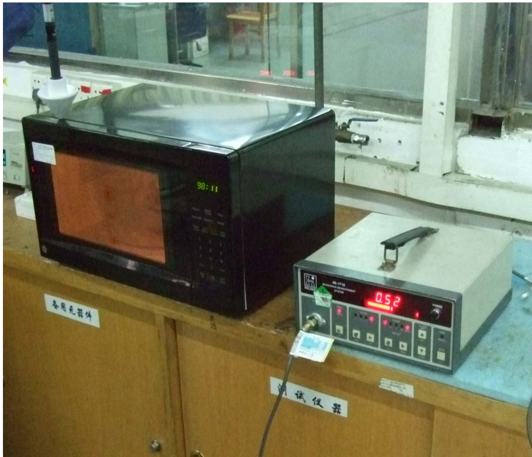
Radiation Hazard Test Setup
