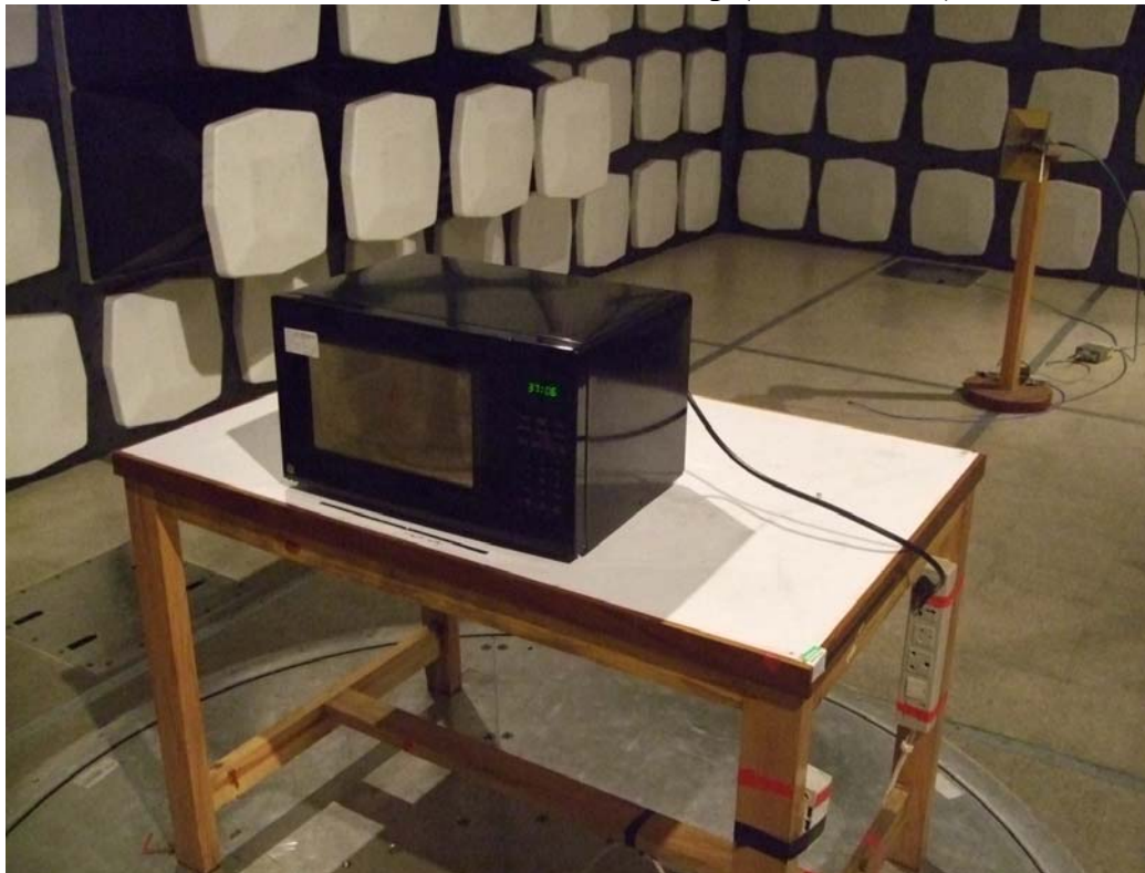
Radiated Emission Test Setup (1-25GHz)
