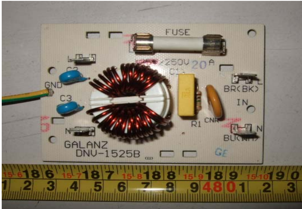
Front View of AC power filter board
