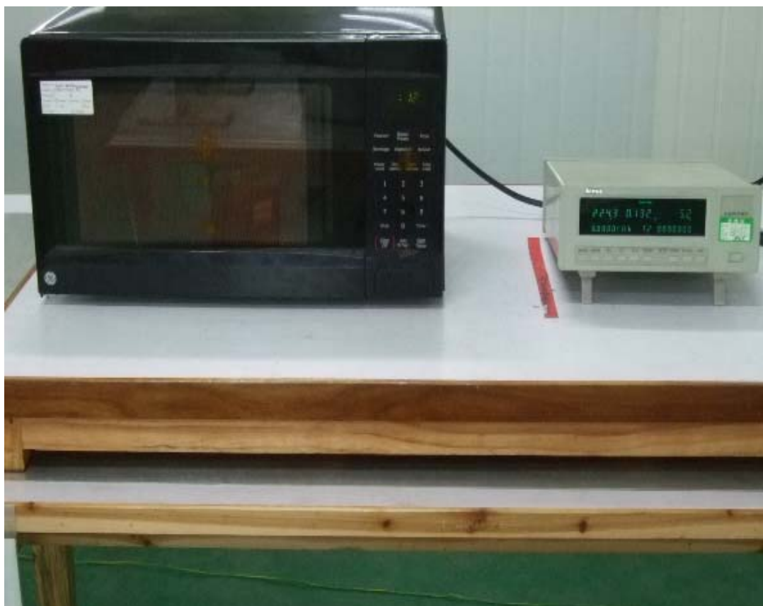
Input Power Test Setup
