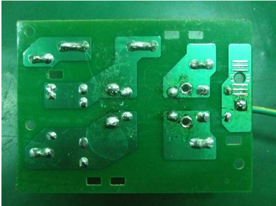
Photo 3 - Back view of AC Power filter board
