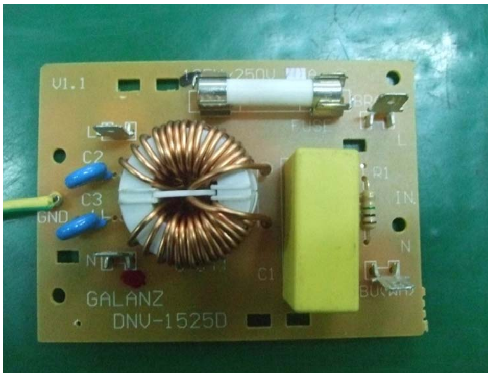
Photo 2- Front view of AC Power filter board
