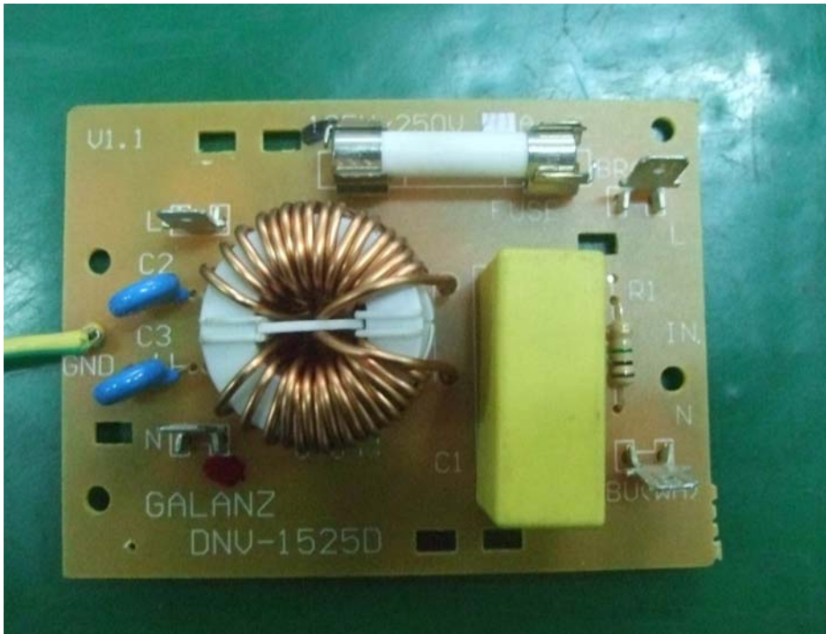
AC power filter board #1
