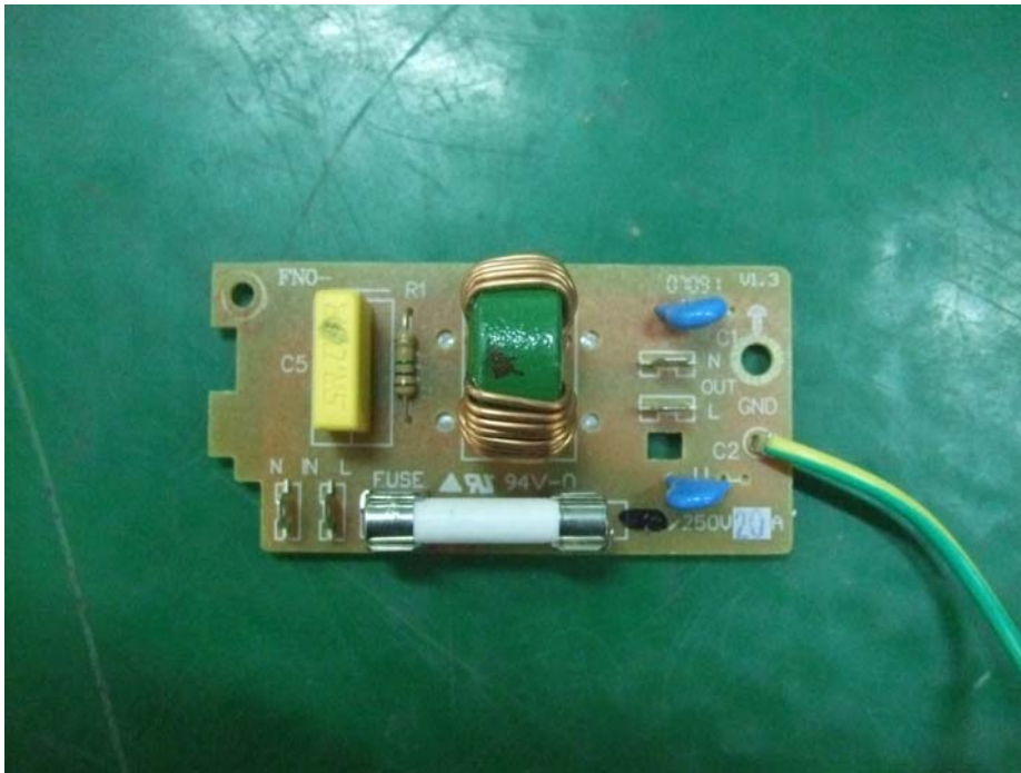
AC power filter board #1
