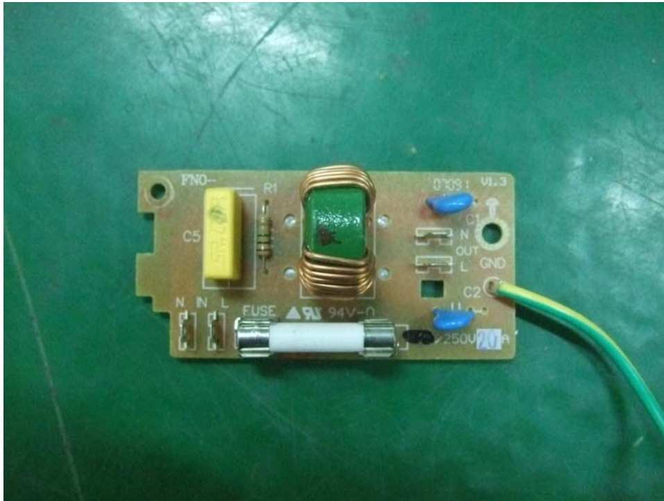
Photo 5 - Front view of Power filter
