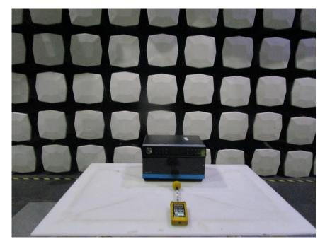
1.6 Operating Frequency Measurement Test Setup
