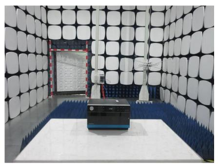
1.4 Radiated Emissions (Magnetic field Strength) (9kHz-30MHz) Test Setup
