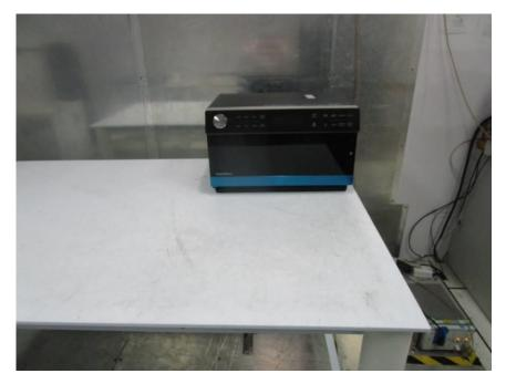
1.2 Radiated Emissions (30MHz-1GHz) Test Setup
